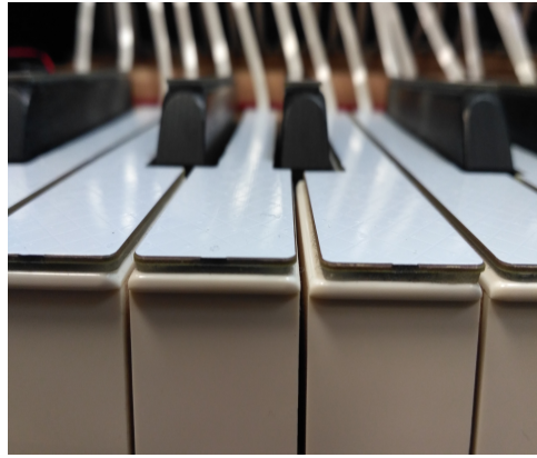
Figure 41: TouchKeys sensors attached on keys
