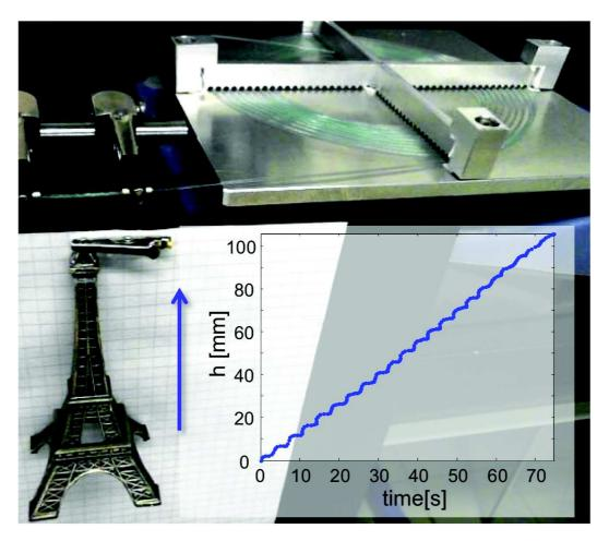
Figure 3.4: Spiral fiberdrive (fiber thickness 0.8mm, total spiral length 3.2m) realized according to the design showed in Fig. 2.10. It is rotating at 185°C lifting a payload (Eiffel Tower replica of weight 20 g). The fiber is guided from the spiral holder through two brass tubes and rotates freely there. Inset: position of the weight as it is lifted.
