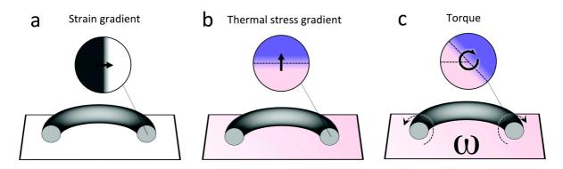
Figure 2.6: a) From its topology, the torus has a strain gradient imposed by the bending. b) When put in contact with a hot plate, the temperature gradient between the surface and the ambiant air induces a thermal prestrain in the z-direction perpendicular to the plane. c) The conflict between the geometrically imposed prestrain and the thermally driven prestrain gives rise to a dynamic instability : the torus begins to turn with a constant speed  $\omega$ .
