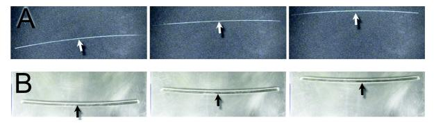
Figure 2.5: Rolling motion of a nylon-6 rod (diameter 0.6 mm, length 12 cm) (A) and a PDMS rod (diameter 3 mm, length 11 cm) (B).
