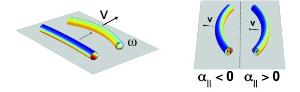
Figure 2.8: The temperature gradient between the hot plate and the ambient air bends the rod via thermal expansion or contraction. Due to the confinement (on the plate) the curving stays in-plane, which effectively creates a torque. The direction of the curvature  $\kappa$  relative to the velocity V depends on the sign of the thermal expansion coefficient.
