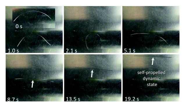
Figure 3.10: Slow annealing of a 800  $\mu$ m nylon fiber at 110°C results in some transient reshaping and eventually within the time course of 10-20 seconds leads to an ideally straight and rolling fiber.
