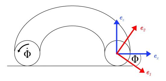
Figure B.1: A fiber confined by its own weight in the X-Y plane. When considering a cross section in the X-Z plane, the curvature can be assumed along the X direction. The co-rotating frame is spanned by the vectors  $e_1$  and  $e_2$ , with the angle  $\Phi$  between  $e_1$  and  $e_2$
