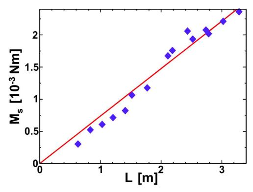
Figure 3.8: The stalling torque of the spirals studied in Fig. 3.7 as a function of spiral length, which displays a linear scaling (red line)
