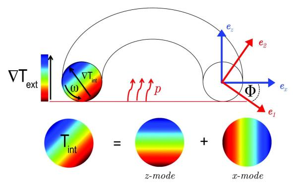
Figure 2.7: The geometry of the toroidal fiberdrive. The internal temperature profile  $T_{int}$  of each cross-section is decomposed in two modes. The thermal z-mode is pumped by the heat flux p normal to the substrate (represented by the red horizontal line). The x-mode  $\Delta T_x$  emerges from the z-mode  $\Delta T_z$  by frame rotation with the angle  $\Phi$ .
