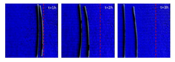
Figure 2.13: Macaroni noodles rolling on the surface of a wet sponge-like material. Pasta is a versatile tool to demonstrate the fiberboid effect. Here it is driven by an evaporation flux. The time scales are four orders of magnitude slower than for the thermal fiberboid but it is nonetheless the same physics that powers the motion.
