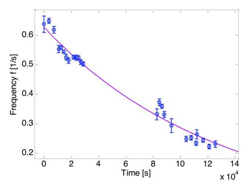
Figure 3.5: Continuous operation long time-testing of a spiral fiber motor. The fiber (nylon-6) is guided to a 13 turn, 0.6 mm diameter spiral and runs at T=160°C. The magenta line is a fit to  $f(t) = f_0 exp(\frac{-t}{t_r})$ , with  $f_0 = 0.63$ Hz and with the exponential frequency relaxation time of  $t_r = 34h$  (1.28x10<sup>5</sup>s). The error bars are the standard deviations from 10 separate measurements.
