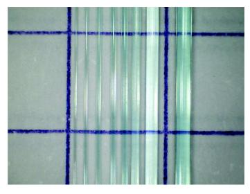
Figure 3.1: The main samples studied are fishing lines made of Nylon with diameters ranging from 0.12mm to 0.8mm.
