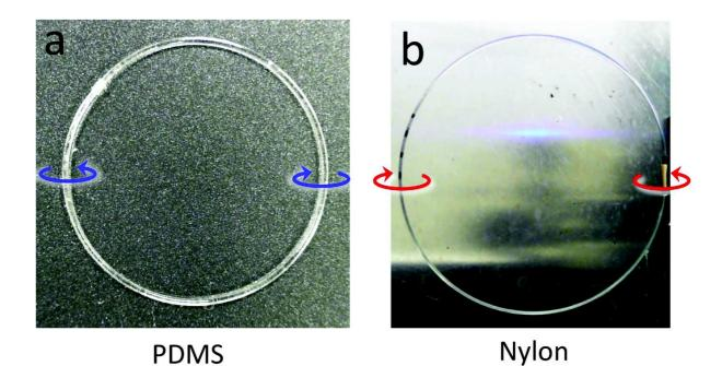
Figure 2.4: Experimental realizations of the fiberdrive with a) PDMS (radius 2cm, thickness 0.6mm) and b) Nylon (radius 6cm, thickness 0.6mm). The direction of rotation depends on the sign of the thermal expansion coefficient, positive for PDMS and negative for Nylon.
