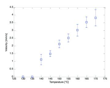
Figure 3.14: Rolling velocity as a function of the plate temperature for annealed PVDF fibers of diameter 0.5 mm. The errors bars are calculated from the standard deviations of ten measurements.
