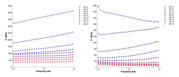
Figure A.1: Mechanical characterization of nylon-6 fibers. Left: The storage modulus vs. frequency for temperatures from 30 to 190°C. Right: The loss modulus vs. frequency for the same temperature range.
