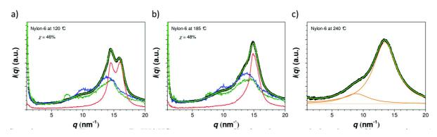
Figure A.3: 1D WAXS intensity profile for the annealed nylon-6 fiber at a) 120°C, b) 185°C, and c) 240°C and the corresponding fitting curve (light green curve). The red (equatorial), blue (45 degrees oblique) and dark green (meridional) curves correspond to the scattering profiles from the sections in Fig. A.2. The orange curves in c) are the amorphous peaks contributing to the signal for the polymer melt.
