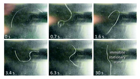
Figure 3.11: Exposing a nylon fiber (800  $\mu$ m) directly to an elevated temperature (180°C) results in rapid uncontrolled reshaping. The final shape remains stationary and does not move or roll over the surface.
