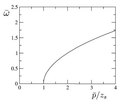
Figure 2.9: Continuous onset of rotation of a fiver closed to a ring as given by (2.22). Shown is the scaled angular velocity,  $\bar{\omega}$ , as a function of the rescaled effective driving  $\frac{\bar{p}}{z_{1}}$ .
