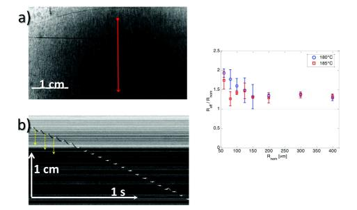
Figure 3.12: Measurement of linear and angular velocity. a) A nylon-6 fiber of radius 60  $\mu$ m rolling at 185°C. b) Kymograph of the motion along the red line in a). In addition to a constant velocity linear motion, the fiber displays a velocity modulation (yellow arrows) in phase with its rotary motion. On the right, the effective radius of the fiber is shown, deduced from the ratio of linear and angular velocity.
