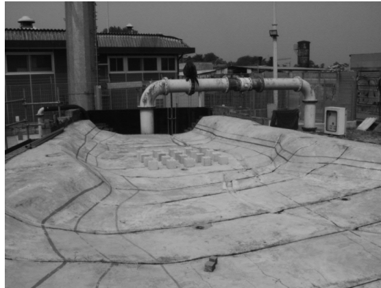
Figure 2.12: Upstream part of the physical model where the model city has been implemented (aligned city layout) (Testa et al. (2007))
