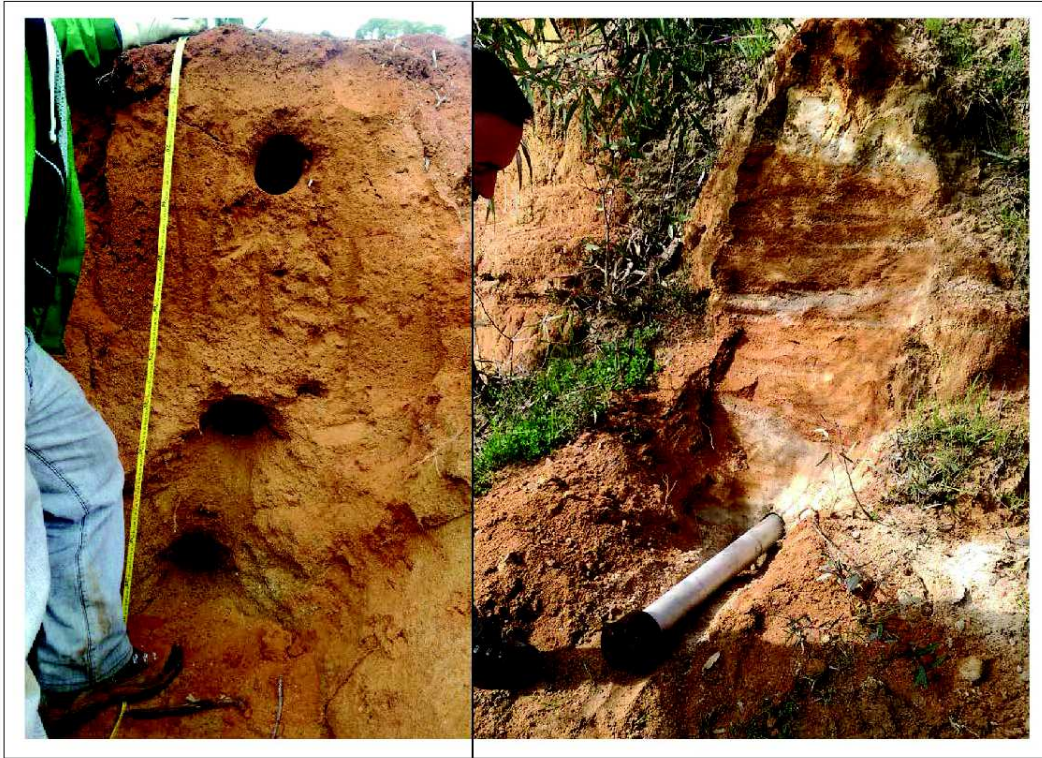
Figure 2-4. Paleochannel sediment deposit profiles showing sampling strategy. Left panel: sampling profile with depth displaying 3 core locations: one at the bottom of the profile; one in the middle of the profile; and one near the surface, Right panel: bottom core sample being hammered in, displaying aluminum core pipe and metal core head.
