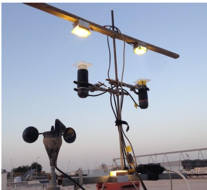
Figure 2. A pair of “outdoor soiling microscopes” (OSMs). Dust particles settle on glass coupons attached to the microscopes, and LED back-lights enable consistent images to be taken day and night
