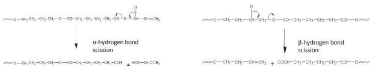
Figure SI 30: Polyester \alpha - and \beta -scission mechanisms
