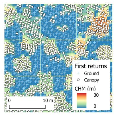
Fig. 5.4 Vertical crown cover from first-returns proportion.
