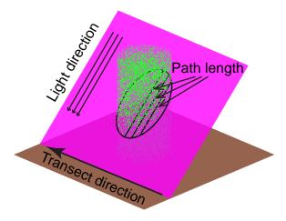
Fig. 3.2 Path length within a cylindrical canopy.
