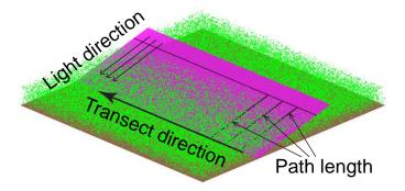
Fig. 3.1 Path length within the homogenous scene.
