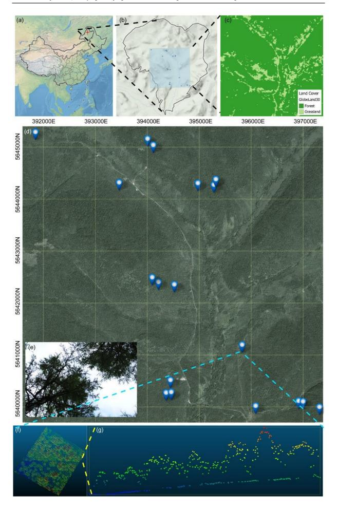
Fig. 5.2 Airborne laser scanner data area and 18 field sites in the Genhe forestry reserve. (a) The position of the research area, (b) Google physical map of the research area, (c) Globeland30 Land Cover map of the ALS data area, (d) Google satellite map of the ALS data area and the positions of the 18 field sites, (e) upward photography and (f) point cloud data of site L1, (g) a transect of the point cloud data of site L1.
