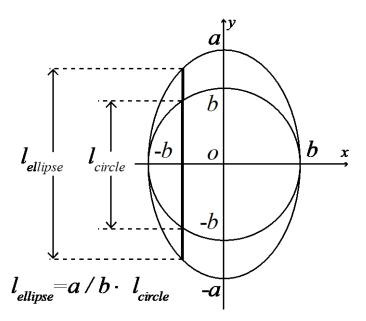
Fig. 3.3 Path length of the ellipse and circle.  $l_{circle}$  is the path length through a circle with a radius of b,  $l_{ellipse}$  is the path length through an ellipse, which is proportional to a circle, and the lengths of semi-major and semi-minor axes of the ellipse are a and b, respectively.
