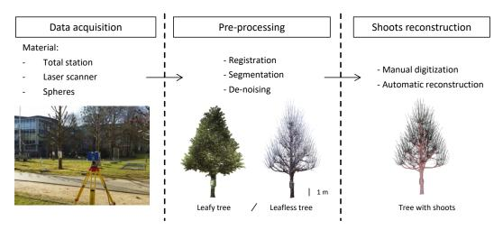
Fig. 4.5 Terrestrial laser scanning data acquisition, pre-processing, and reconstruction of the studied tree (Source : E. Bournez).
