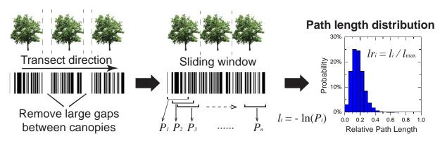
Fig. 3.4 Flow of obtaining path length distribution from measured gap data.  $P_i$  is the gap probability in each window,  $l_i$  is the path length in each window,  $l_{max}$  is the max path length along the transect, and  $lr_i$  is the relative path length in each window.
