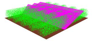
Fig. 3.5 Overview of the cylindrical row canopy scene. Disk-shaped leaves with a radius of 0.05 m are colored green, soil ground is colored brown, and observing angles are represented by pink planes.
