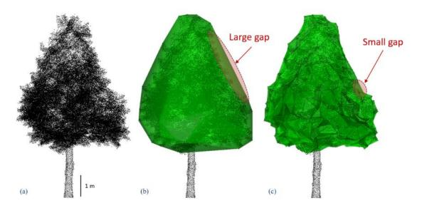
Fig. 4.7 The merged point cloud (a), convex envelope (b), and concave envelope (c) of the studied tree crown.
