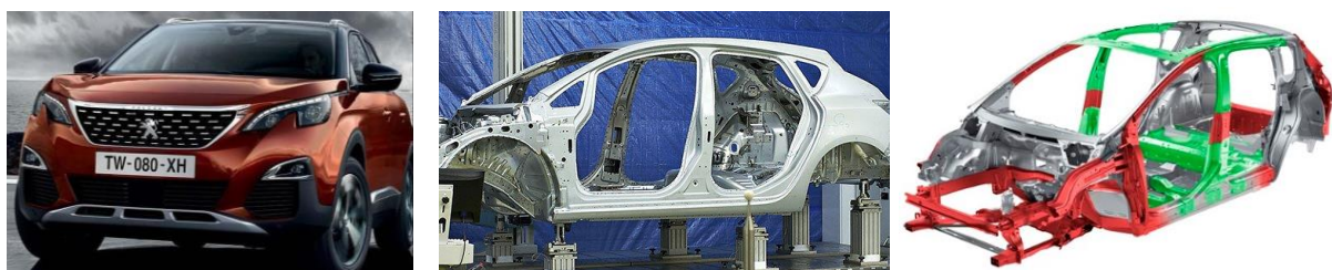
Figure G.3: 3008 series Peugeot automobile: a) finished car, b) its BiW, partially incorporating fibre-reinforced material in the metal framework, and c) coloured image of the same BiW to represent different structural parts (red: steel, green: aluminium)[G.10-G.11].
