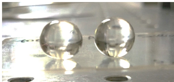
Figure 55. Samples of water retaining SPA polymers in the bubble shape.
