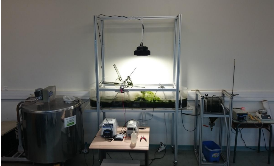
Figure A 9 HRAP system operation (high light condition).
