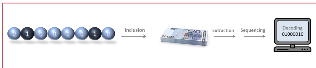
Figure 7: Schematic representation of the use of sequence-defined polymers as anti-counterfeiting taggants for materials labeling
