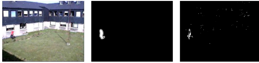
Figure 3.37: On the left and at the middle are sample input and ground truth images respectively from the 2014 CDnet dataset, PTZ category. To the right is the image produced by SOM-QE on detecting the changes between the input image and its next image frame on the video. The PTZ category of images posed unique challenges on change detection, with other methods in the literature managing F1 score of less than 0.30. SOM-QE scored an F1 score of 0.39, which is the best score in this category.
