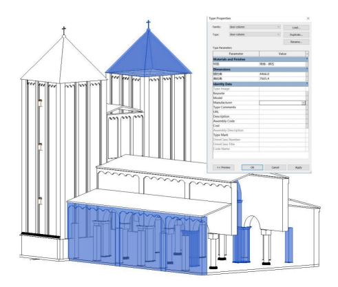
Figure 5.10. The final parametric HBIM model of the Abbey of Niedermunster in 3D views with parametric geometry and extensible properties
