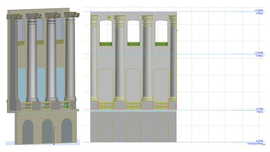
Figure 3.22. The point clouds are manually transferred to parametric model
