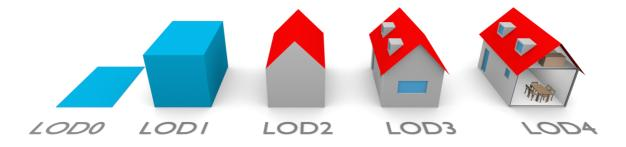
Figure 3.4. Building models in LOD0-LOD4 (image from Biljecki et al., 2016)
