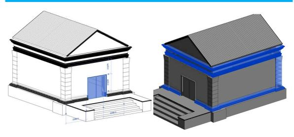
Figure 5.9. The final parametric HBIM model of the Petit château du Meisenbach in 3D views, whose parameter and semantic information can be modified further
