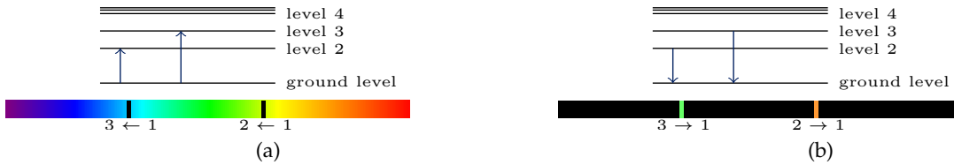
Figure 1.2: (a) Absorption and (b) emission spectra.
