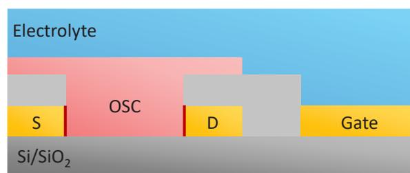
**Figure IV.16** Staggered structure for the suppression of the crowding effect. The SiO<sub>2</sub> layer covers the whole top surface of source and drain. The injection and detection areas are pointed out with the dark red lines.
