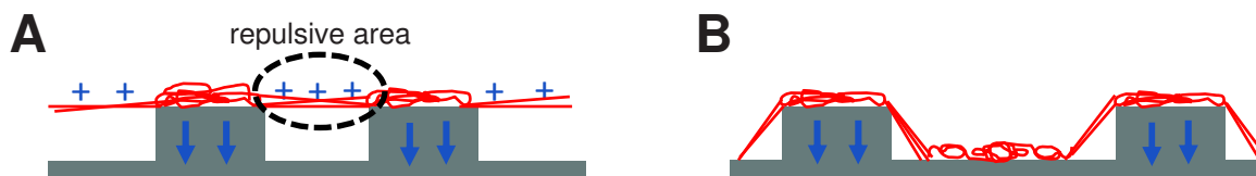
Figure 5.2. Schematic representation of fibers deposition on conductive blocks. (A) When height/distance is high, fibers stay hanged over the holes and charges are not dissipated. (B) When height/distance is low, fibers deposit on the flat area of the collector between the blocks. Blue arrows indicate the dissipation of the charges through the collector.
