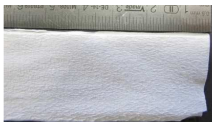
Figure 5.20. Picture of a membrane made of aligned PLA fibers and pPGS/HP \beta CD particles.
