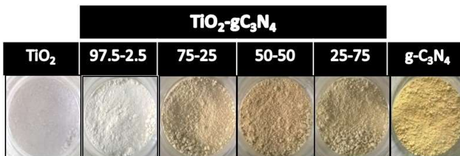
Figure 4.27. Comparison of the color in function of g-C 3 N 4 content of all (screening and zoom) TiO 2 (NTs)-gC 3 N 4 composites and references.
