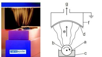
Principle of needleless electrospinning
