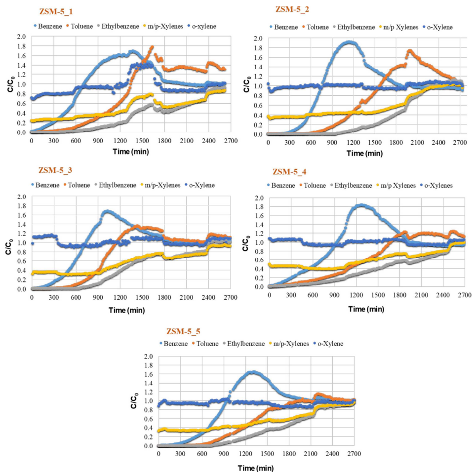
Fig. 2. Breakthrough curves obtained during BTEX adsorption experiments with 10 ppm mixture.
