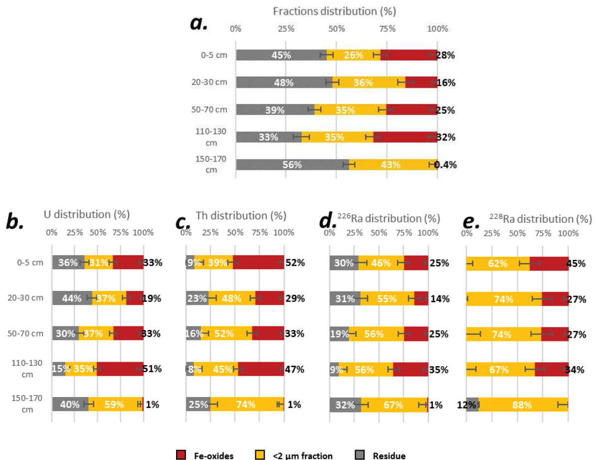
Figure 3-7 : Proportions of the separated soil fractions and distribution of U, Th and Ra isotopes within these fractions. The fraction distribution was estimated by solving the system of Eq. 1.
