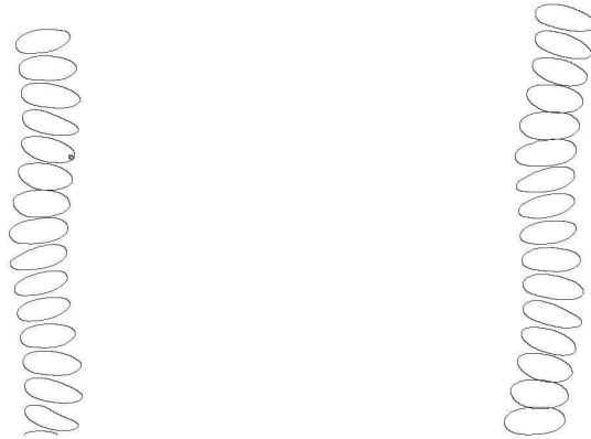
FIGURE 5.8: Bubble helical path in two orthogonal planes XZ (left) YZ(right) at Bo=10 and Ga = 94 in silicon oil 10cst
