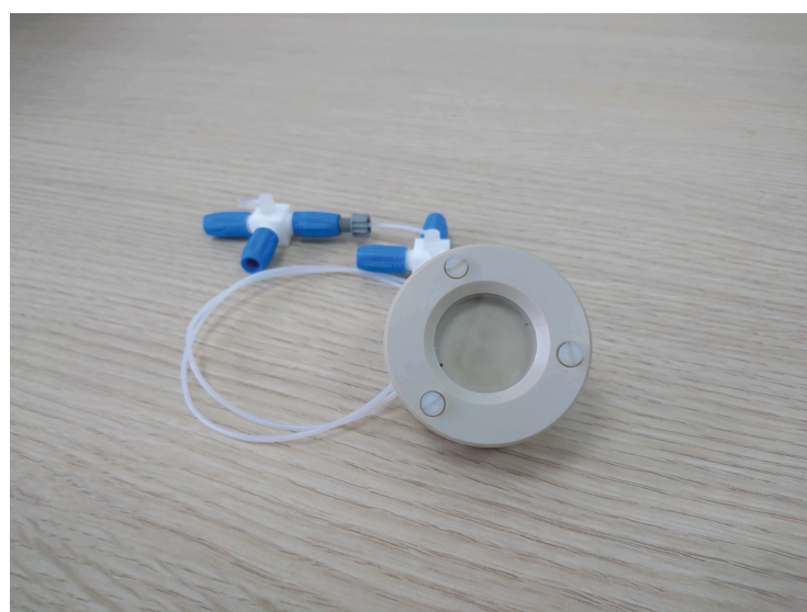
Figure II.2.12 – Solid/liquid cell for fluorescence microscopy experiments.
