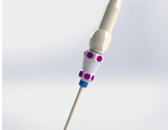
FIGURE 3.8: Design of the LED ring assembly mounted on the laparoscope handle
