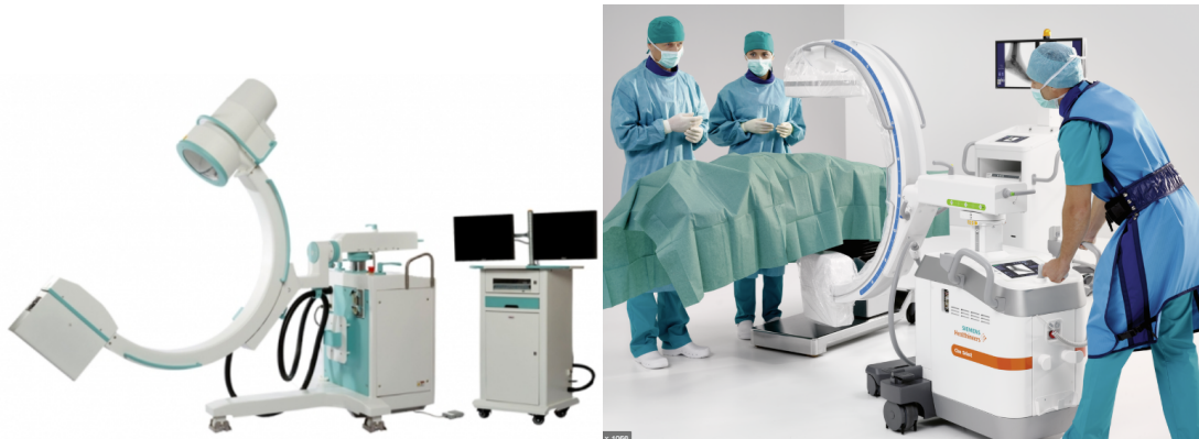
FIGURE 2.6: Left: C-arm imaging machine (Image from www.kiranxray.com ). Right: C-arm machine during a surgery (Image from www.siemens-healthineers.com )
