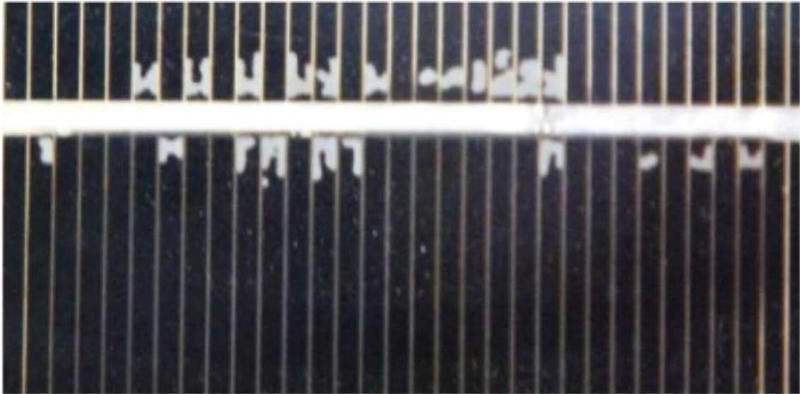
Fig. 45 Delamination at the cell-EVA interface in the proximity of the interconnection ribbons.
