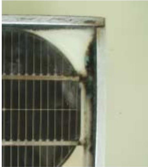
Fig. 44 Water penetration in a 21-year-old PV panel caused by backsheet detachment.
