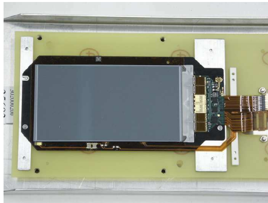
Figure 2.9: Single-sided TIB module. The 512 strips are read-out by 4 APV chips on the right-hand side. Taken from Ref. [158].
