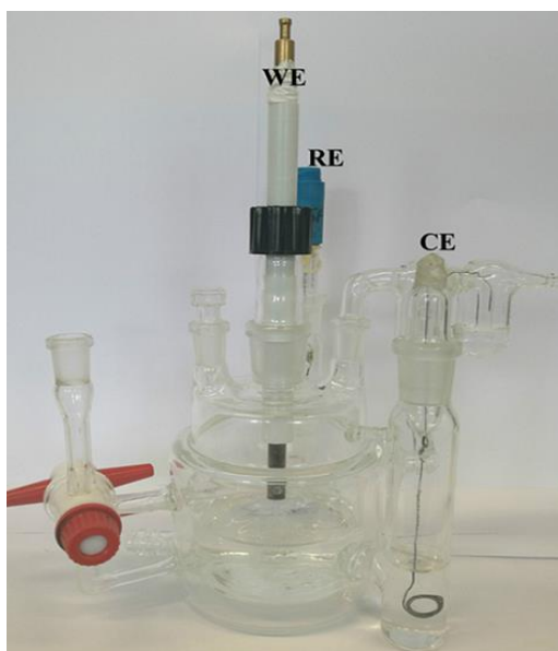
Fig. 2-5. Three-electrode glass cell system.
