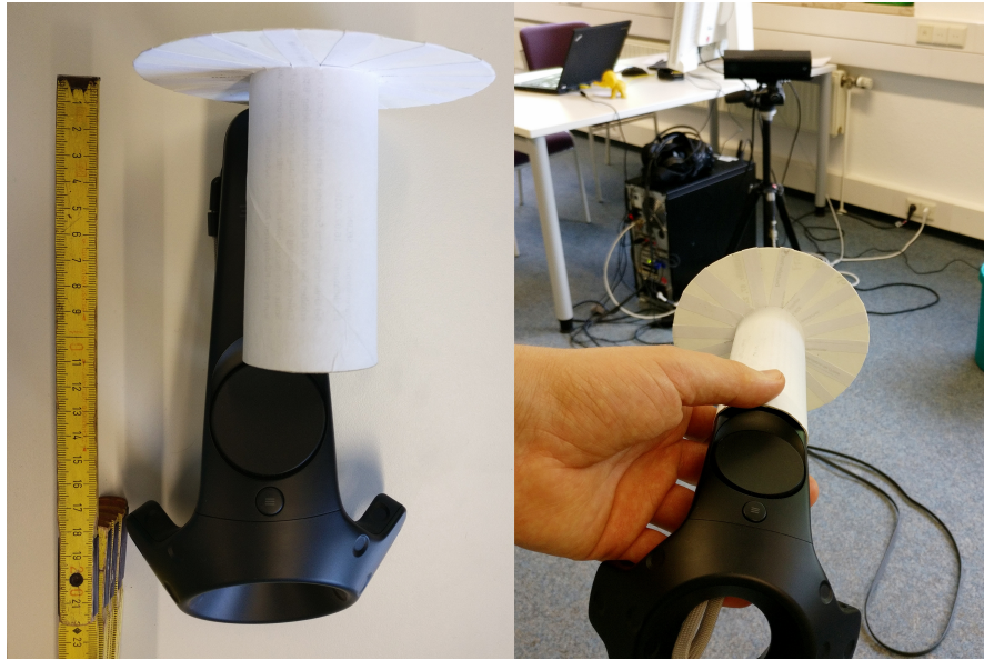
Figure 3.9 Vive controller with mounted disc target.
