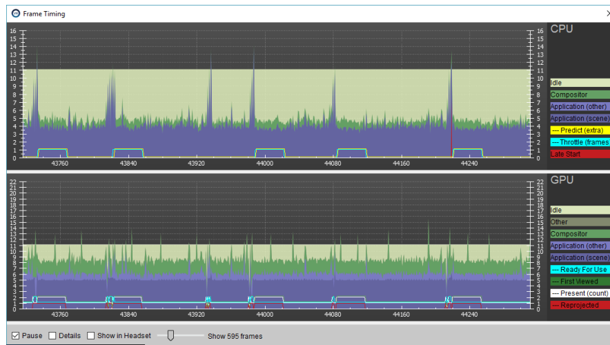
Figure 3.7 The rendering times for a Kinect 2 point cloud using the native program library concept of Unity are on average less than 11ms.
