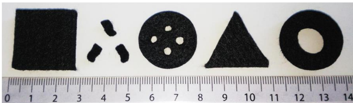
Figure 3. Graphite felts with different macroscopic shapes for various catalytic applications both in gas- and liquid-phase processes.
