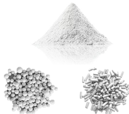
Figure 13. The main forms of synthetic zeolites (powder, ball, extenders)
