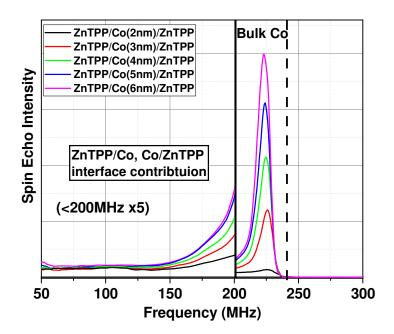
**Figure 9:** Evolution of FNR spectra for Cu/Fe/ZnTPP(20ML)/Co (t in nm)/ZnTPP(20ML)/Fe samples with the increase of Co thickness from 2nm to 6 nm. Measurements are conducted at 1.8K, sample surface area is of  $3cm^2$ , spectral intensity below 200 MHz are magnified by a factor of 5 (x5).
