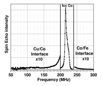
**Figure 12:** FNR spectrum of a typical Cu/Co/Fe sample. Low radiofrequency (< 200MHz) range corresponds to the Cu/Co interfacial contribution. High frequency range (> 240 MHz) corresponds to the Co/Fe interface contribution.
