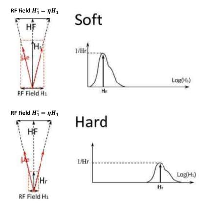
**Figure 8:** A schematic representation of the rf field enhancement process: applying the radiofrequency field  $H_1$  results in the oscillation of the electronic magnetization  $\mu_e$  which in turn results in the oscillation of the  $H_{HF}$ . The oscillation of  $H_{HF}$  then leads to the resulting radiofrequency  $H_1^*$  that is sensed by the probed nuclei. The figure is taken from ref. [111].
