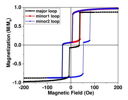
**Figure 8:** Magnetic simulations showing the major and minor magnetization loops for the Cu(25nm)/Fe(30nm)/ZnTPP(20ML)/Co(5nm)/ZnTPP(20ML)/Fe(30nm) hybrid system. Both minor magnetization loops show positive shift with an exchange field of +27 Oe. All magnetization loops are normalized to saturation magnetization.
