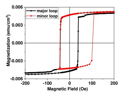
**Figure 9:** Major and minor magnetization loops for 100nm Cr capped Cu(25nm)/ZnTPP(20ML)/Co(5nm)/ZnTPP(20ML)/Fe(30nm) heterostructure. The minor loop shows a shift towards the positive field axis with an exchange field of 32 Oe. For all loops, the measurements are at 2K.
