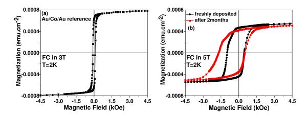
**Figure 3**: Magnetization loop of (a) 10nm capped Au/Co(6nm) reference sample, FC in +3T (b) "freshly deposited" Co(6nm)/ZnTPP(10nm)/Au(10nm) hybrid sample (black loop) and the same sample measured again after 2 months (red loop). Hybrid samples' loops are acquired at 2K after FC in +5T.
