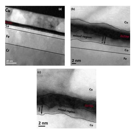
**Figure 18:** (a) (b) (c) Dark field STEM images for Cu/ZnTPP (20ML)/Co/Fe/Cr heterostructure. The different layers are separated by black contours for clarity. In (b) and (c) the imaging is focused on the ZnTPP/Co interfacial areas. Mixed regions are of 3nm-3.5nm thick, extended into the molecular film.
