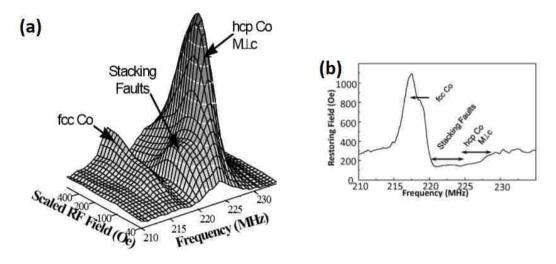
**Figure 9:** (a) 3D FNR spectrum in a hcp cobalt single crystal. The FNR signal intensity is represented as a function of frequency and scaled radiofrequency field  $H_1$  (b) The plot representing the restoring field as a function of resonance frequency. The figures are taken from ref. [111].
