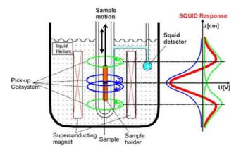
**Figure 4:** The interior components of SQUID magnetometer. The maximum/optimum SQUID output voltage signal is detected when the sample is well situated in-between the blue pick-up coils. The figure is taken from ref. [97].
