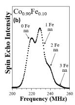
**Figure 11:** FNR spectrum of (a) Co-Cu (b) Co-Fe. In all spectra,  $0 \times 10^{-2}$  X nn ( $X = 10^{-2}$  Cu or Fe) means no alien metal atom within the 12 NN cell of cobalt i.e. cobalt sees only cobalt atoms in its environment. 1, 2, ... X nn ( $X = 10^{-2}$  Cu or Fe) corresponds to the replacement of 1,2... Co atoms in the NN cell by alien elements. The figures are taken from ref. [111].
