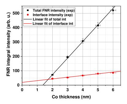
**Figure 10:** Estimated integral intensities of the FNR spectra of figure 5. Red and black symbols are the experimental data obtained for total and bulk part integral intensities and their respective solid lines (red and black) represent the linear fits.
