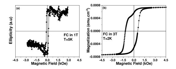
**Figure 6**: Magnetization loop of (a) "freshly deposited" Co(10nm)/CoTPP(10nm)/Au(10nm) hybrid sample measured via MOKE. Loop acquired at 5K after FC in 1T (b) same sample measured again after 2 months this time with SQUID. Loop acquired at 2K after FC in +3T external magnetic field.
