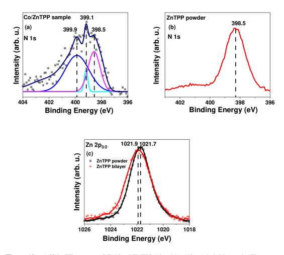
**Figure 10:** (a) *N* 1*s* XP spectra of Co(6nm)/ZnTPP(10nm)/Au(10nm) hybrid sample. The dark blue spectrum is the cumulative fitted spectrum from the three other spectra present in the same plot. (b) *N* 1*s* XP spectrum for ZnTPP compounds (c)  $Zn 2p_{3/2}$  XP spectra of ZnTPP compound (black) and Co(6nm)/ZnTPP(10nm)/Au(10nm) hybrid sample (red).
