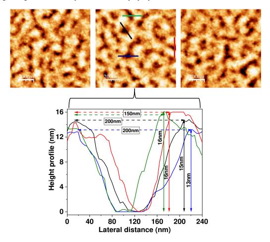
**Figure 11:** Top panel: Surface images of the 50nm Au capping layer on top of Au(25nm)/Co(6nm)/ZnTPP(10nm) stack. The images are acquired with AFM using tapping mode in ambient condition. The 3 images correspond to different zones of the same sample. Scan area is of  $1\mu m^2$ . Bottom panel represents the height profiles of the respective line profiles (color codes on the image) extracted from the middle image.
