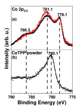
**Figure 9:** Co  $2p_{3/2}$  XP spectra of (a) Au(25nm)/Co(6nm) uncapped reference sample (black spectrum) and of Co(6nm)/ZnTPP(10nm)/Au(10nm) hybrid sample (red spectrum), (b) Co(II)TPP compound. Scattered plots are the raw data and the bold lines are the smoothened spectra. The shake-up satellite peak is present at 786.3 eV for all spectra, and it results from the multi electron excitation process during a photoemission mechanism.
