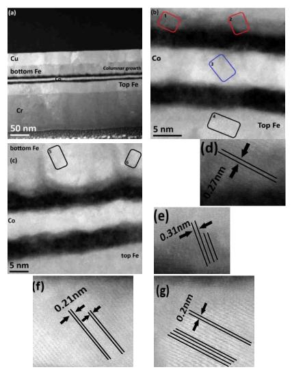
**Figure 16:** (a) (b) (c) Dark field STEM images for Fe/ZnTPP/Co/ZnTPP/Fe sandwich sample. Bottom iron shows columnar growth. Red rectangular boxes are for the fringes in the mixed iron-ZnTPP interface. Blue box for the fringes in the cobalt film while the black boxes corresponds to the fringes in top and bottom iron layers. (d) (e) (f) (g) inter-planar distances for the boxes marked as 1, 2, 3 and 4, respectively.
