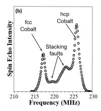
**Figure 10:** FNR spectrum of (a) Dominant fcc cobalt structure, with weaker hcp contribution at higher frequency and peaks corresponding to the stacking faults in-between. The spectrum above 219 MHz is magnified (x5) for visual clarity. (b) Dominant hcp cobalt with fcc and stacking fault contributions observed at lower radiofrequency range. The figures are taken from ref. [111].
