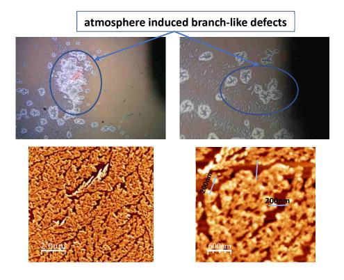
**Figure 14**: Top panel: AFM camera images of the surface defected ZnTPP film of the Au(25nm)/Co(6nm)/ZnTPP(10nm) sample. Branch-like structures are observed and can be differentiated from the intact zones. Bottom panel: AFM scan images at 10 micron (right) and 3 micron (left) of the degraded samples. The spaces between one structure and the other extend up to 200nm (marked by the gray profile on the bottom right image).
