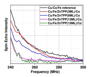
**Figure 6:** Evolution of FNR spectra with increasing thickness of the ZnTPP layers on Fe. The high radiofrequency contributions (> 240 MHz) decrease with the increase in ZnTPP thickness and vanish at 15 ML. Only high radiofrequency spectral range is represented in the plot. Measurements are at 2K.
