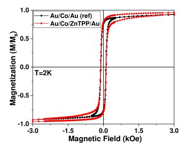
**Figure 2:** Black curve: Magnetization loop of Au(25nm)/Co(6nm)/Au(10nm) reference sample, FC in +3T magnetic field. Red curve: Magnetization loop of the "freshly deposited" non-aged Au(25nm)/Co(6nm)/ZnTPP(10nm)/Au(50nm) hybrid sample, FC in +6T magnetic field. The loops are acquired at T=2K and are normalized to saturation magnetization.
