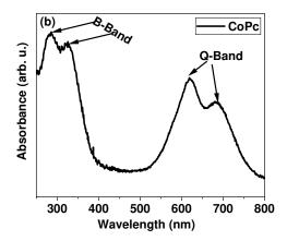
**Figure 3:** UV-Visible spectrum of (a) Zn(II)TPP, Ni(II)TPP and Co(II)TPP molecular films (b) CoPc molecular film. All molecular films are 10nm and are deposited on quartz glass substrate.
