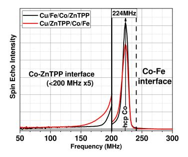
**Figure 11:** Spectra for Cu/Fe/Co/ZnTPP (black) and Cu/ZnTPP/Co/Fe (red) heterostructures. The low frequency spectra region is magnified by a factor of 5 (x5). Co-ZnTPP interface corresponds to the contribution from Co/ZnTPP and ZnTPP/Co type of interfaces.
