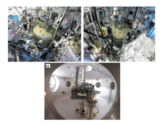
**Figure 2:** (a) and (b) top view picture of the "Hybrid" system. 2- load lock chamber, 3- robot-arm chamber, 4- sputtering chamber, 5- evaporation chamber, 6- OMBE chamber. (c) the interior of the robot-arm chamber with the valve gates of the evaporation (5) and OMBE (6) chambers. The pictures are taken from ref. [96].
