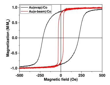
**Figure 2:** Magnetization loops of Au(evap)/Co(10nm)/Au(10nm) (black hysteresis) and Au(e-beam)/Co(10nm)/Au(10nm) (red hysteresis) measured with AGFM at room temperature in an external magnetic field of 1000 Oe.
