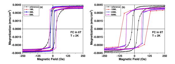
**Figure 4:** Magnetization loop of (a) Cu/Co(6nm)/Fe(30nm) reference sample (black curve) and Cu/Co(6nm)/ZnTPP(t)/Fe(30nm) heterostructures with ZnTPP thickness of 1ML, 3ML and 6ML (b) Cu/Co(6nm)/Fe(30nm) reference sample (black curve) and Cu/Co(6nm)/ZnTPP(t)/Fe(30nm) heterostructures with ZnTPP thickness 15ML, 24ML and 60ML. All the heterostructures are capped with 100nm of Cr. All loops are measured at 2K after FC in in-plane +6T external magnetic field.
