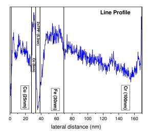
**Figure 13:** Profile of the line plot in figure 14. Estimated thicknesses are consistent with the deposited thicknesses.
