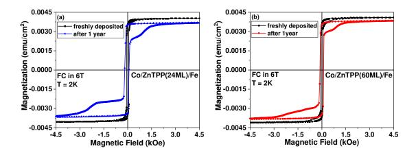
**Figure 1:** Magnetization loops of (a) Cu(25nm)/Co(6nm)/ZnTPP(24ML)/Fe(30nm) sample. Black loop: directly after growth, blue loop: measured again after 1-year (b) Cu(25nm)/Co(6nm)/ZnTPP(60ML)/Fe(30nm) sample. Black loop: directly after growth, red loop: measured again after 1-year. The two samples are capped with 100nm of Cr. All loops are measured at 2K after FC in an in-plane +6T external magnetic field.
