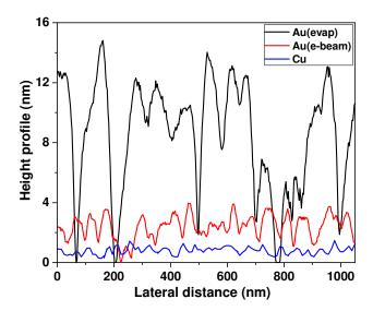
**Figure 2:** The height profiles of the surface for the different buffer layers. Black: Si/SiO<sub>2</sub>/Au(evap), Red: Si/SiO<sub>2</sub>/Au(e-beam), and Blue: Si/SiO<sub>2</sub>/Cu. The thickness of the buffer layers is 25nm for all samples
