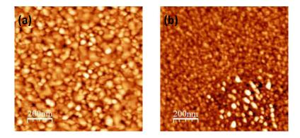
**Figure 1:** Surface morphology of (a) 25nm of Au(e-beam) seed layer (b) 25nm of Cu buffer layer deposited on Si/SiO<sub>2</sub> substrate. Cu buffer layer shows smoother and more uniform surface morphology compared to Au layer.
