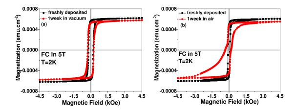
**Figure 5**: Magnetization loop of (a) "freshly deposited" Co(6nm)/NiTPP(10nm)/Au(10nm) hybrid sample (black loop) and the same sample measured again after 1 week, while kept in vacuum (red loop) (b) "freshly deposited" Co(6nm)/NiTPP(10nm)/Au(50nm) hybrid sample (black loop) and the same sample measured again after 1 week, while exposed to air (red loop). Magnetization loops are acquired at 2K after FC in +5T external magnetic field.
