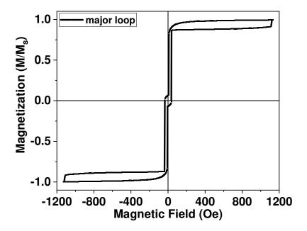
**Figure 7:** Magnetic simulation of the major hysteresis loop for Cu(25nm)/Fe(30nm)/ZnTPP(20ML)/Co(5nm)/ZnTPP(20ML)/Fe(30nm) heterostructure. It is calculated using the model described in the text. The magnetization curve is normalized to saturation magnetization.
