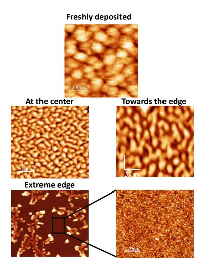
**Figure 15:** Top panel: free surface morphology of NiTPP film of Au(25nm)/Co(6nm)/NiTPP(10nm) sample. Scan size is  $1\mu m^2$ . Middle and bottom panel: AFM scan images of surface degraded Au(25nm)/Co(6nm)/NiTPP(10nm) sample acquired at the center  $(2\mu m^2)$ , towards the edge  $(1\mu m^2)$  and extreme edge  $(1\mu m^2)$ . Bottom right panel is the image for molecule-free area  $(1\mu m^2)$ , showing a molecule-free surface with  $\sigma_{RMS} = 0.15nm$ .
