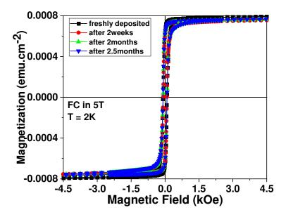
**Figure 3:** Magnetization loops of Au(25nm)/Co(6nm)/ZnTPP(10nm)/Cr(100nm) sample. Same sample has been measured 4 times, over a period of 80 days. Between each measurement, sample is kept in a desiccator. All measurements are done at 2K after field cooling in +5T external magnetic field.
