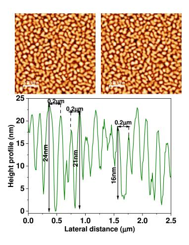
**Figure 12:** Top panel: AFM surface images of the 10nm capping Au layer on top of Au(25nm)/Co(6nm)/ZnTPP(10nm) stack, scanned at 3μm scan size. Bottom panel: The height profile of the surface, extracted from an arbitrary zone. The profile shows the cracks to be 200nm wide and have depth ranges between 16nm to 25nm. Scans are conducted at ambient conditions.
