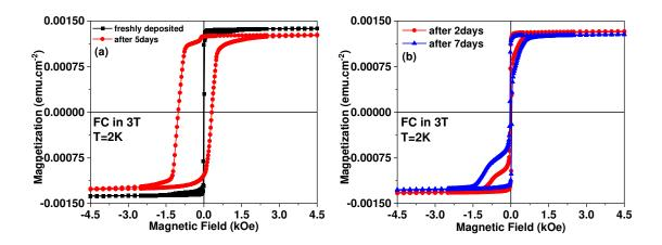
**Figure 7**: Magnetization loop of (a) "freshly deposited" Co (10nm)/CoPc(10nm)/Au(10nm) hybrid sample (black loop) and of the same sample measured again after 5 days (red loop). (b) already aged Co(10nm)/CoPc(10nm)/Au(50nm) hybrid sample measured after 2days (red loop) and measured again after 7days (red loop). Magnetization loops are acquired at 2K after FC in +3T external magnetic field.
