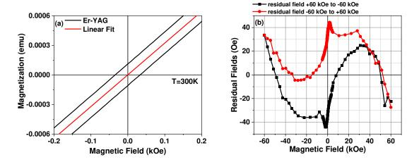
**Figure 5:** (a) black: magnetization curve of the Er:YAG sample, red: linear fit of the measured magnetization curve. The graph is scaled at [200 Oe, -200 Oe] for the details of the low field region. (b) Evolution of the residual fields of the SQUID as a function of applied magnetic field.
