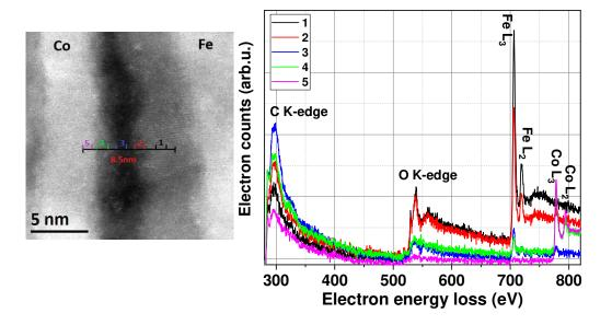
**Figure 15:** (left) Dark field STEM survey image for EELS spectroscopy. (right) EELS spectra acquired from the line profile of the survey image. Each spectrum corresponds to its number and color code, respectively. The integration length to extract the spectrum was of 1nm for each region.
