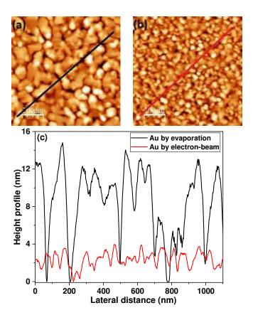
**Figure 1:** Surface image of Au buffer layer prepared by (a) thermal evaporation (b) electron-beam. Scan area is of  $1\mu m^2$ . (c) Height profile of the respective lines (color codes on the images) extracted from the AFM images.
