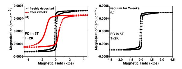
**Figure 4**: Magnetization loop of (a) "freshly deposited" Co(6nm)/ZnTPP(10nm)/Au(50nm) hybrid sample (black loop) and the same sample measured again after 2 weeks (red loop) (b) "fresh but old" Co(6nm)/ZnTPP(10nm)/Au(50nm) sample, kept in UHV for 2 week. The magnetization loops are acquired at 2K after FC in +5T external magnetic field.
