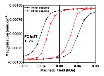
**Figure 8**: Magnetization loops of 10 nm capped Co/CoPc (black curve) and 50 nm capped Co/CoPc (red curve) after being in UHV chamber for 5 days before measurement. The samples are not exposed to atmosphere, until time of measurements. Loops acquired at 2K after FC in +3T.
