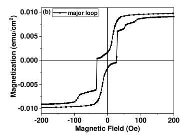
**Figure 5:** (a) Major magnetization loop at T=2K for the 100nm Cr capped Cu(25nm)/Fe(30nm)/ZnTPP(20ML)/Co(5nm)/ZnTPP(20ML)/Fe(30nm) heterostructure
