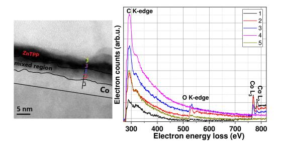
**Figure 19:** (left) Dark field STEM survey image for EELS spectroscopy. (right) EELS spectra acquired from the line profile of the survey image. Each spectrum corresponds to its number and color code, respectively.
