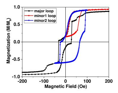
**Figure 6:** Major and minor magnetization loops for the 100nm Cr capped Cu(25nm)/Fe(30nm)/ZnTPP(20ML)/Co(5nm)/ZnTPP(20ML)/Fe(30nm) heterostructure. Both minor loops show a shift towards the positive field axis with an exchange field of +36 Oe. All loops are acquired are at 2K. All magnetization loops are normalized to saturation magnetization value.
