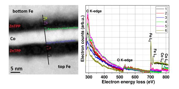
**Figure 17:** (left) Dark field STEM survey image for EELS spectroscopy. (right) EELS spectra acquired from the line profile of the survey image. Each spectrum corresponds to its number and color code, respectively.
