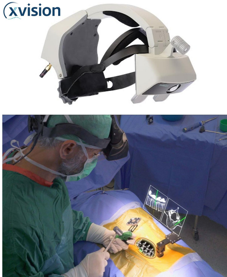
Fig. 1.8. Augmedics xvision™ augmented reality guidance system for surgery and an image of implantation during spine procedures.
