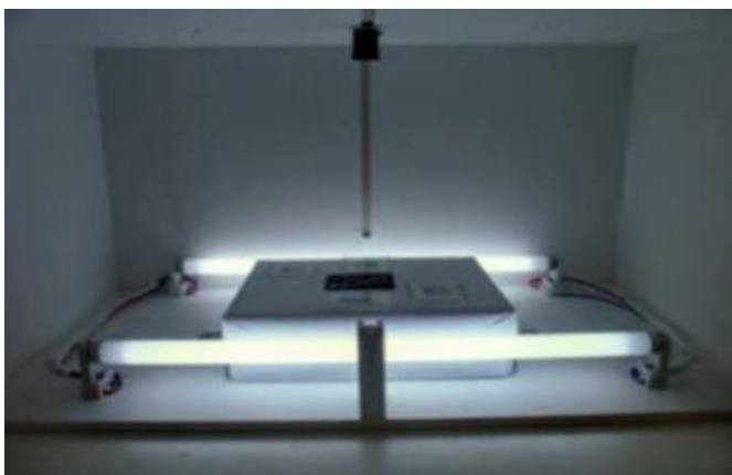
Figure 5.2-4: Photo of the Cycling box created by Ynvisible® to monitor the durability of the ECDs.
