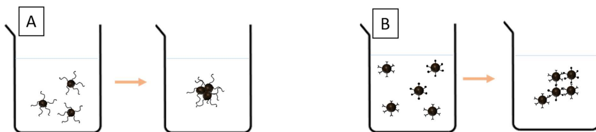
Scheme 5. Controlled assembly of functionalized NPs. A. By insufficient ligands on the surface. B. By interaction between the ligands.
