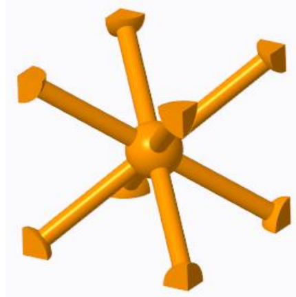
Fig.77: Representation of a regular beam-based lattice structure.
