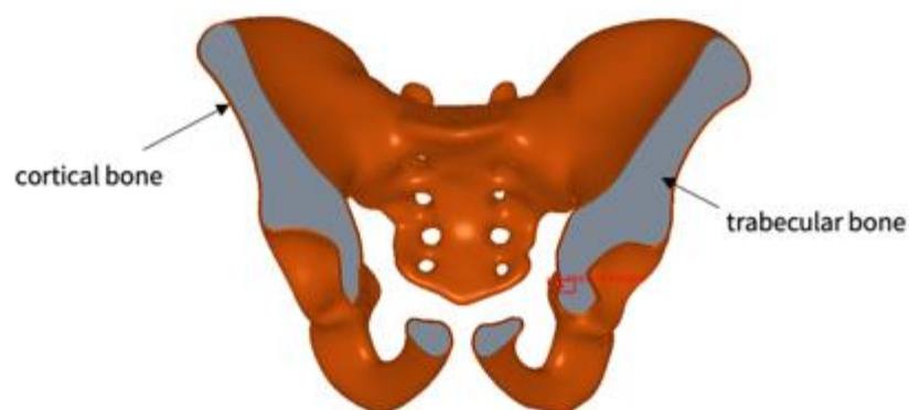
Fig.59: Numerical model of the pelvic bone for the FEA ([Harrer 2020]).
