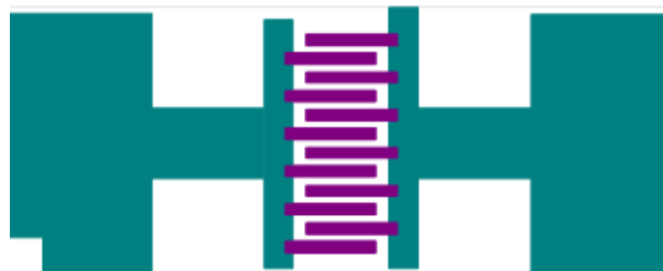
Figure 4-3. Illustration of interdigitated electrode for AuNPs-TEG network based strain sensor. (Green and purple colors stand for different layers; channel length: 5 or 10 \mu\text{m} )
