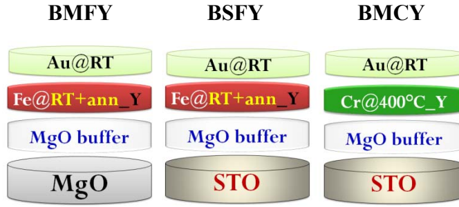
Figure IV- 5: Architecture of Fe buffer layers on MgO(100) and STO(100). The Cr buffer layer was deposited only on STO(100).
