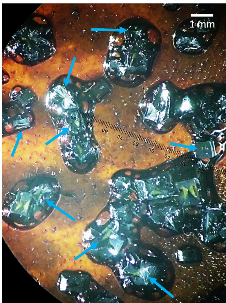
Figure 6.6: Optical image of type-II crystals under white light. The blue arrows point to the hidden crystals which are difficult to see due to their small size or optical shadows from incident light
