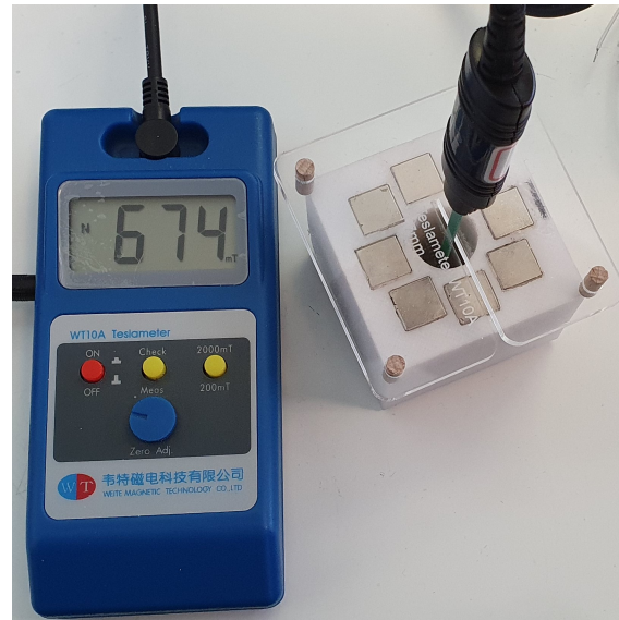
Figure 3.11: The Halbach magnet on the right and the WT10A magnetometer with 1mT resolution on the left.
