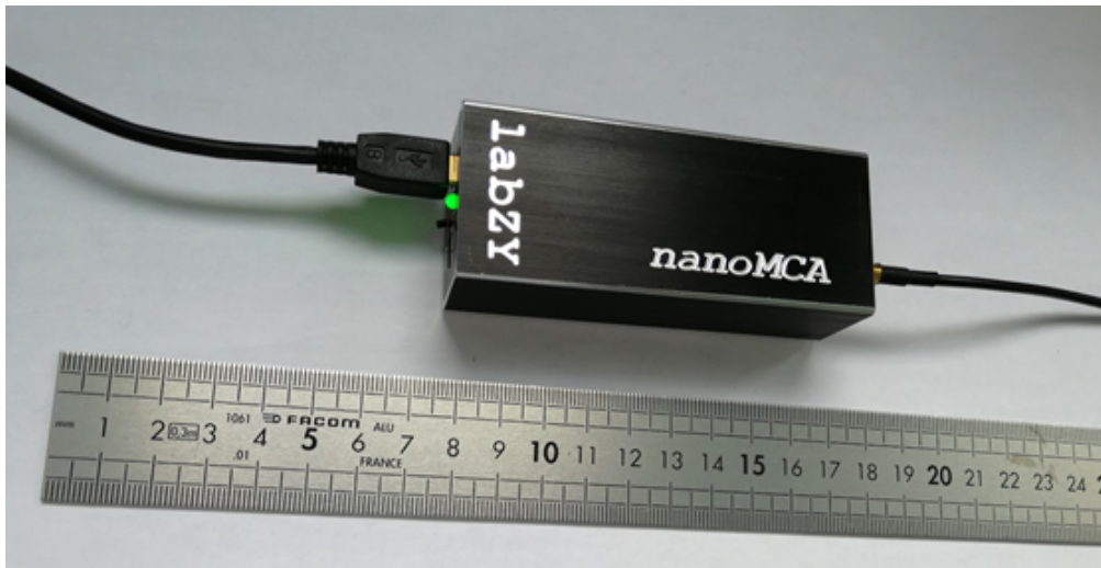
Figure 2.22 – The nanoMCA module from labZY .
