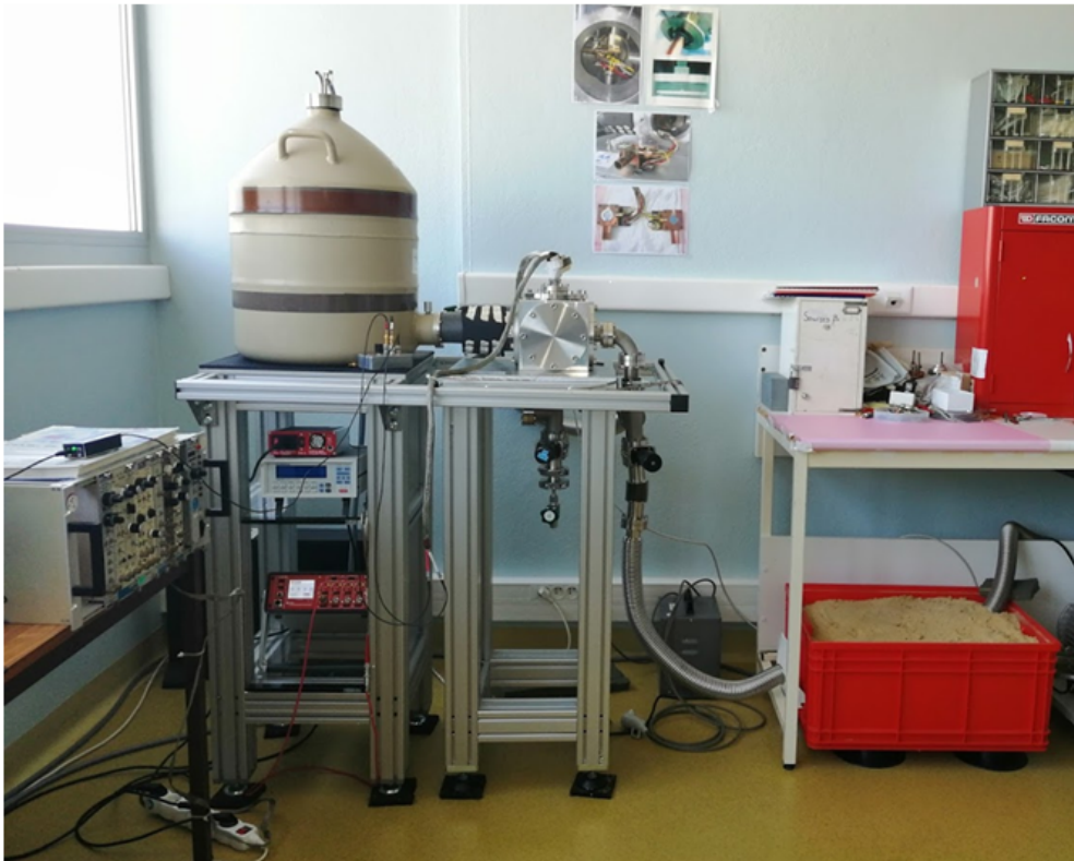
Figure 2.11 – Picture of the new experimental set-up of \beta spectrometry.
