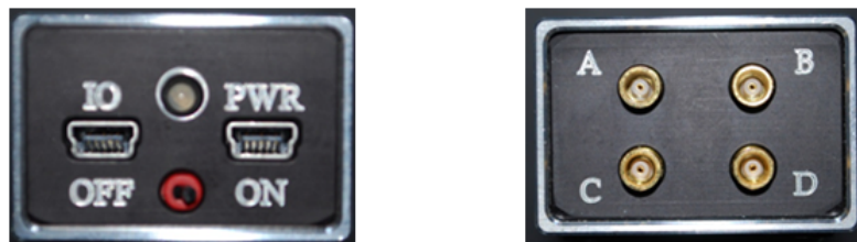
Figure 2.23 – Front (left) and back (right) panels of the nanoMCA module.
