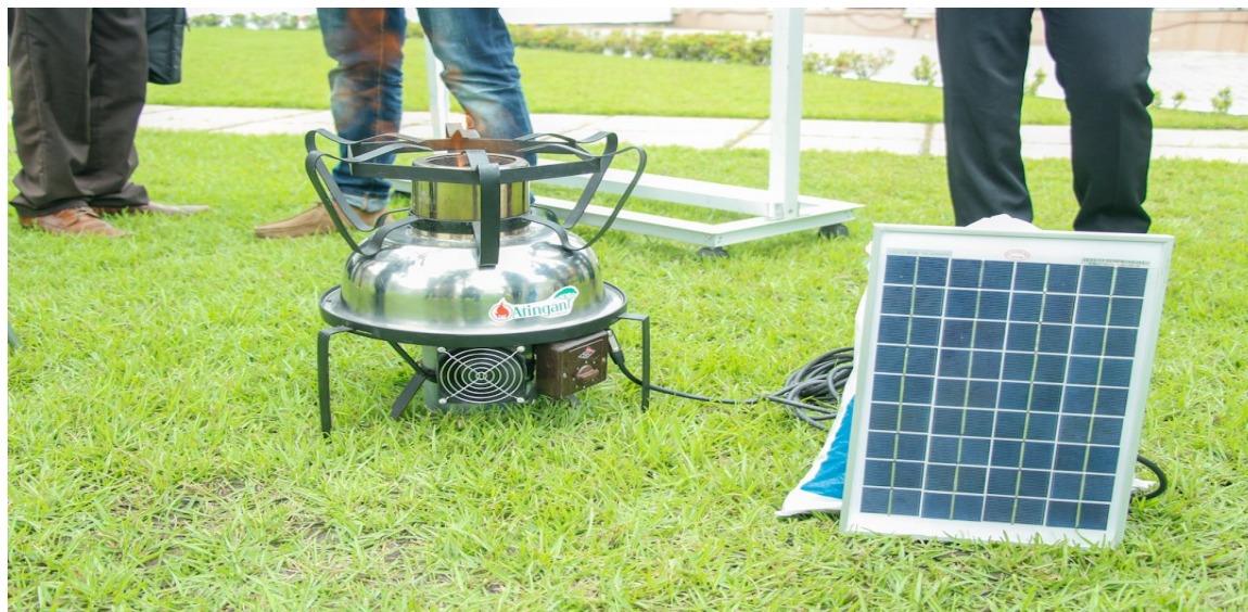
Photo 18 : Foyer hybride solaire-biomasse "Atingan"
