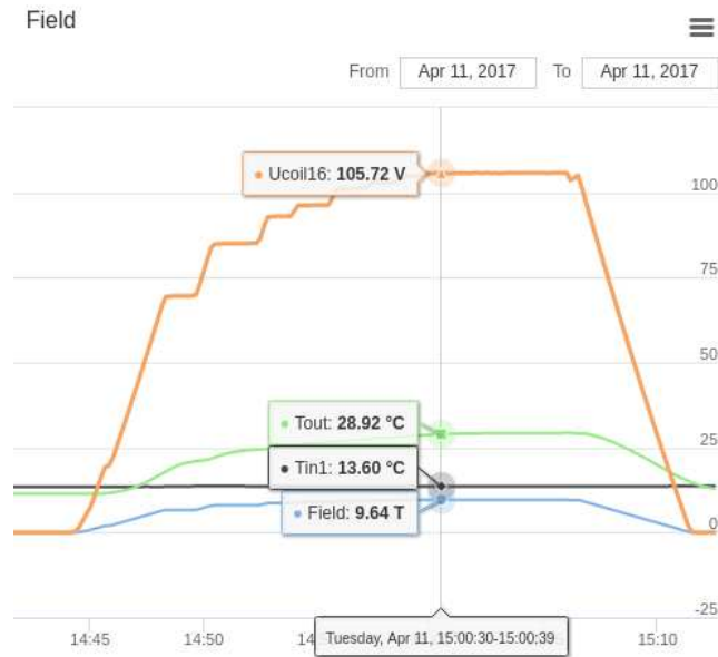
(b) Logs of magnet monitoring system
