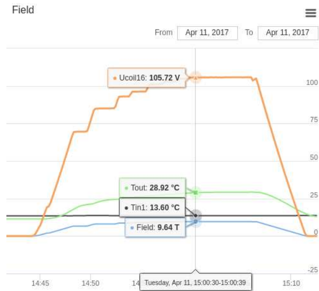
(b) Logs of magnet monitoring system
