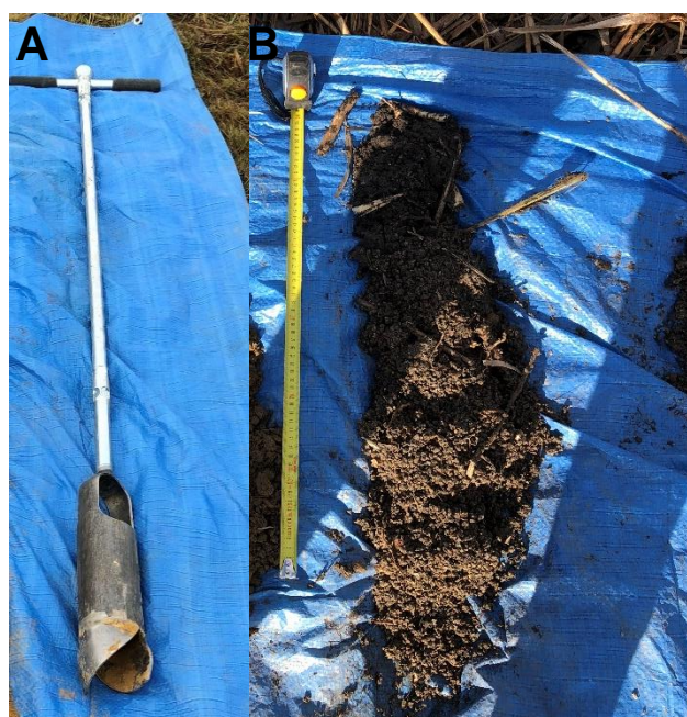
Figure 28: Coring performed in the CW. A) Manual auger used for the coring. B) CW mud vertical profile reconstructed after coring.
