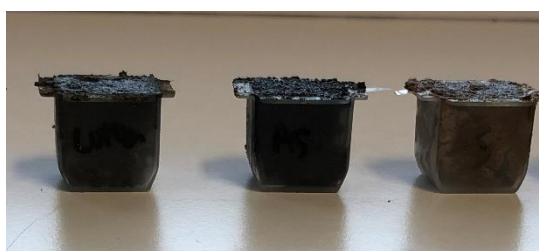
Figure 53: Sludge samples placed in bucket with similar size used for MSI experiments.
