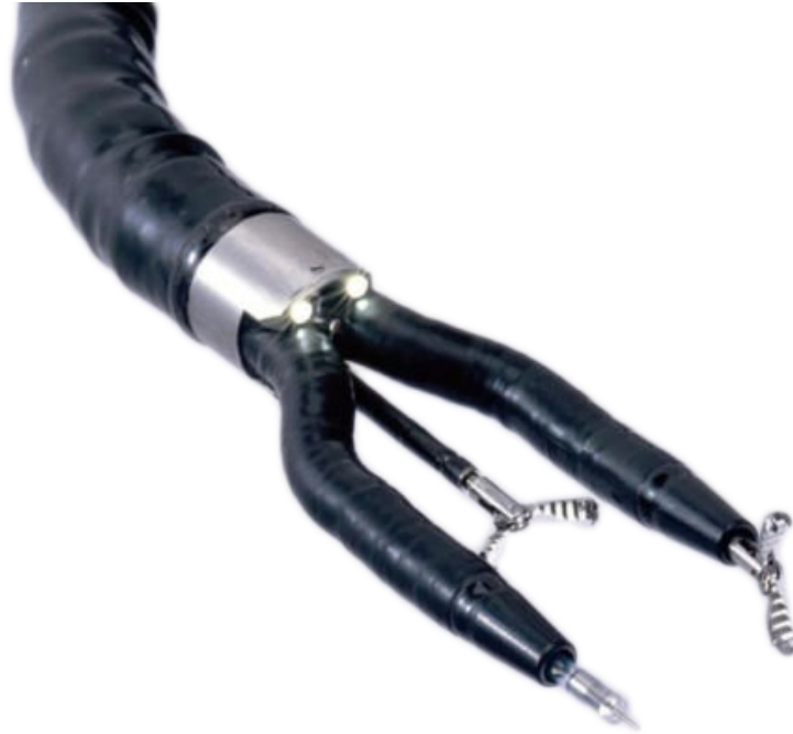
Figure 1.12: View of the distal part of the endoSAMURAI and its flexible arms [Hussain, 2015].
