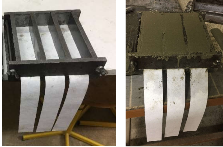
Figure 2- 19: Placement of non-woven sheets in prisms
