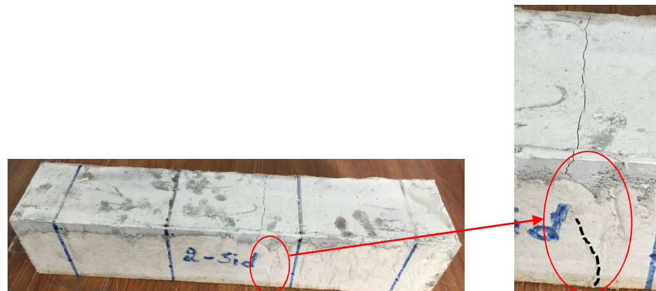
Figure 5- 10: Cracking patterns of beam (2-Sides)
