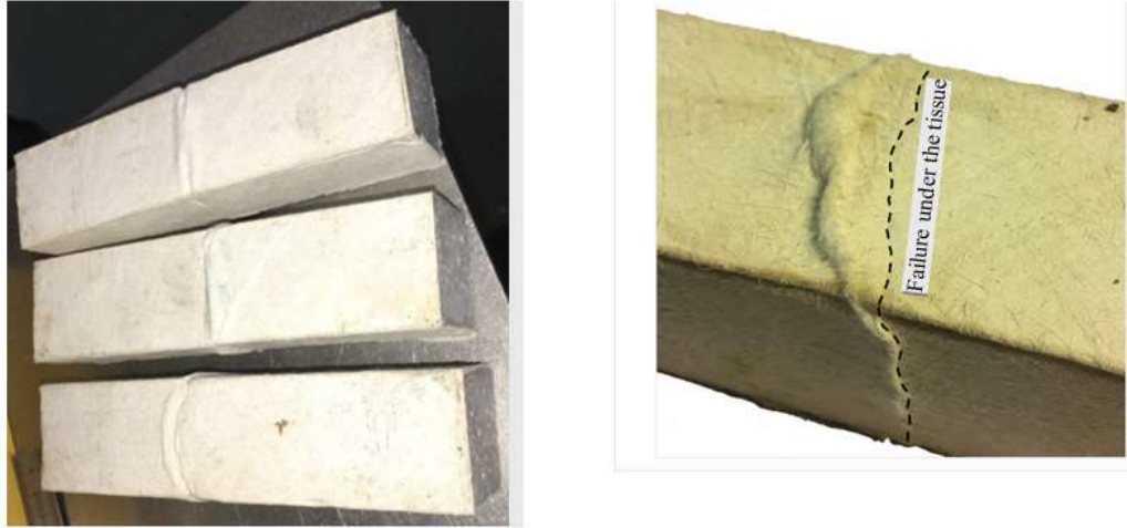
Figure 4- 10: Cracking patterns of mortar prisms (3-Sides)
