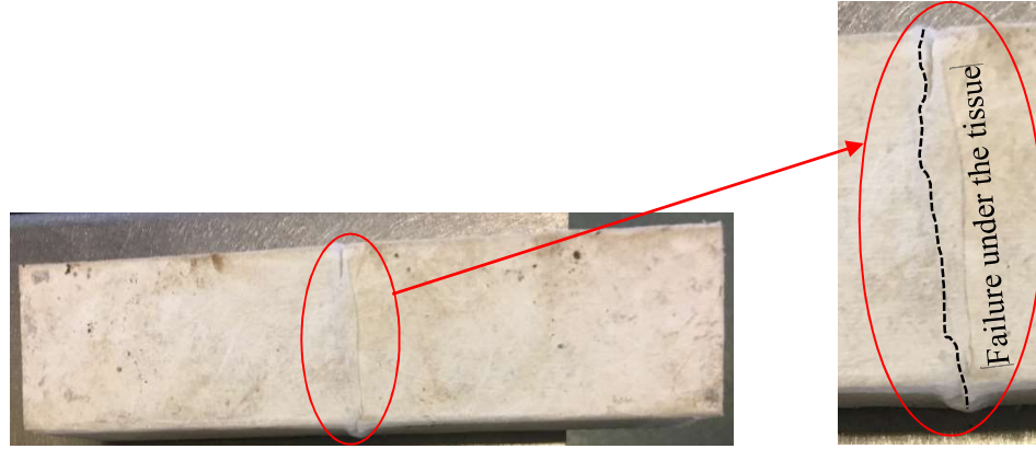
Figure 5- 11: Cracking patterns of beam (3-Sides)
