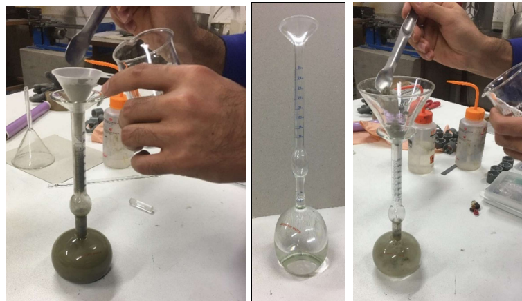
Figure 1: Test procedure for specific gravity of cement
