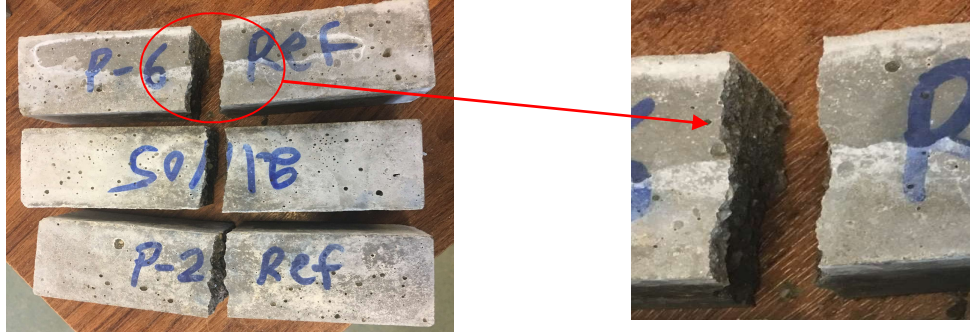
Figure 4- 5: Cracking patterns of mortar prisms (Ref)
