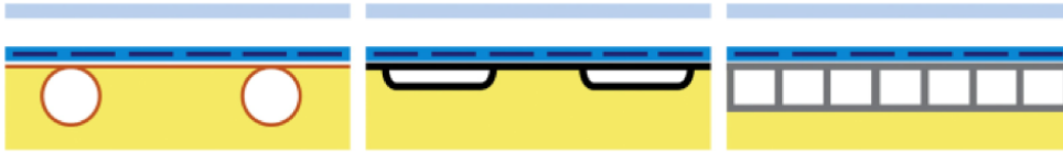
FIGURE 2.22: Tubular, trapezoidal and rectangular channel collector [28]
