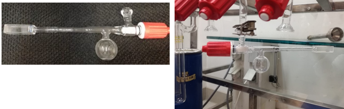
Figure 6.5 Homemade quartz cuvette equipped with a RotaFlo stopcock ( left ) and then attached to the freeze-pump-thaw ( right ).
