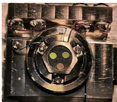
Figure 2.8. Photograph of the sample holder used to fix the cells for the TEMPO beamline.
