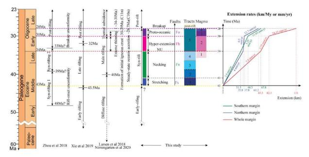
**Figure II.10.** Time frame for the evolution of rifting in the NW-SCS linking regional studies with the tracts, magmatic units, faults and extension rates based on the results of quantification of the restoration shown in Fig. II.8.
