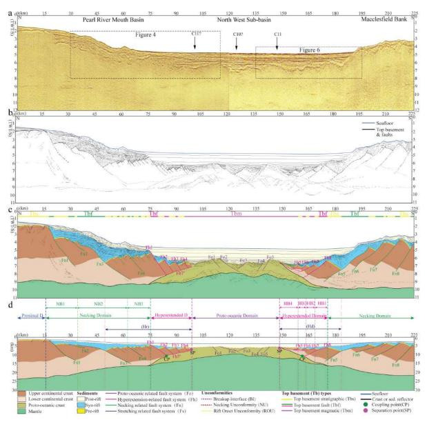
**Figure II.2.** CGN-1 reflection seismic section across the NW-SCS. For location see Fig. II.1. (a) Time migrated reflection seismic section CGN-1. (b) Line drawing of the seismic section CGN-1. (c) Seismic interpretation of CGN-1. (d) Interpreted CGN-1 section with a time to depth conversion.
