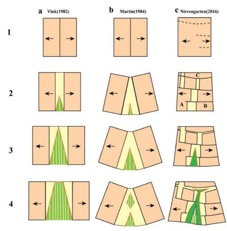
*Figure I.12* Rift propagation models: (a) model from Vink (1982), (b) model from Martin (1984), and (c) model of rift and seafloor spreading of a three-plate system modified from Nirrengarten et al. (2018).
