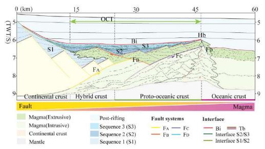
*Figure III.10.* Cartoon showing a schematic representation of the nature and characteristic structures of the crust in the OCT and their link to the sedimentary sequences and magmatic additions. The section summarizes the main observations described from sections CGN-1, 2, 3 and 1555.
