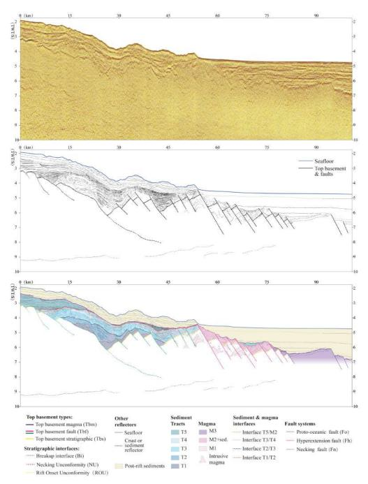
*Figure II.5.* (a) Reflection seismic line CGN-1A located 4 km west of CGN-1 line (see Fig. II.1). (b) Line drawing of the section shown in (a) and interpretation of T1 to T5, Bi and Tb.
