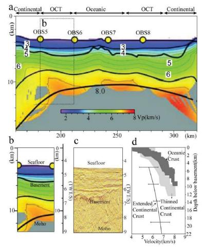
Figure III.8. (a) The OBS2006-1 refraction seismic section from Ding et al. (2012). The OBS2006-1 section is located east of the CGN-3 line (for location see Fig.
