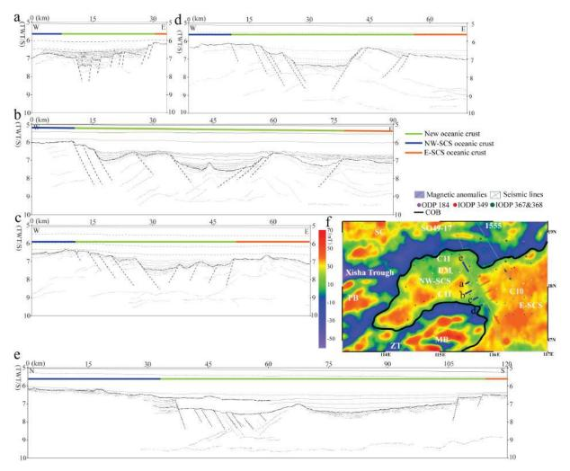
*Figure VII.5.* Extensional tectonic and crustal accretion at oceanic transform faults. (a-d) Line drawing of seismic section across the transform fault. (e) Line drawing of seismic section parallel the transform fault. (f) Free-air gravity anomaly map with location of seismic sections.
