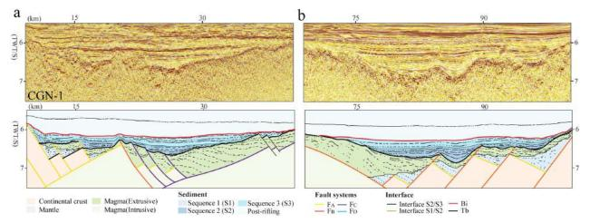
*Figure III.6.* (a) Zoom on CGN-1 line showing the sedimentary architecture of the northern margin. Section below shows line drawing and interpretation of seismic section. (b) Zoom on CGN-1 line showing the sedimentary architecture of the southern margin and line drawing and interpretation in underlying section. For location of zooms see Fig. III.2a.
