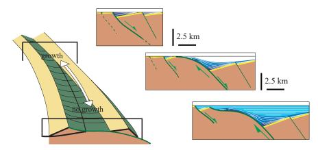
**Figure II.3.** Along strike change of rift and sediment architecture from a highangle normal fault to a down-ward convace long offset detachment fault (modified after Péron-Pinvidic et al. 2007).
