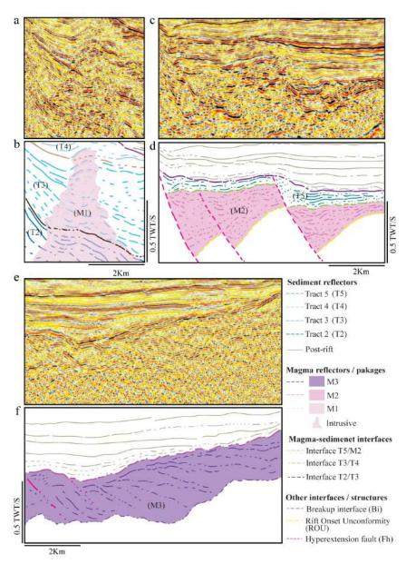
*Figure II.7.* Zooms showing magmatic additions (for location see Fig. II.4a). (a) Seismic detail of magmatic unit 1 in the necking zone and (b) line drawing. (c) Seismic detail of magmatic unit 2 in the hyperextended unit and (d) line drawing. (e) Top magmatic basement in the proto-oceanic domain with oceanward dipping reflections onlapped by sediments of tract 5 and (f) line drawing.
