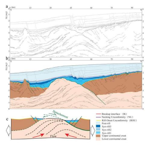
**Figure VII.4.** The lower crustal flow during crust necking. (a) Line drawing of the seismic section come from Baiyun Sub-basin, North SCS. (b) Interpretation of the seismic section. (c) Cartoon model show the evolution and processes linked to necking and the formation of necking unconformites.
