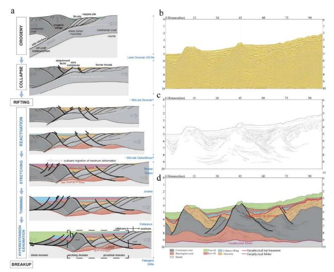
*Figure VII.6.* (a) Schematic representation of the structural evolution of the crust from an orogenic context to a rift. Modified from Peron-Pinvidic et al. (2020). (b-d) An uninterpreted, line drawing and interpreted section of the time migrated reflection seismic section across the Jinghai Sub-basin, in the N SCS.
