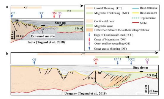
*Figure I.4* (a) Magma-poor rifted margin: seismic observations from the SE Indian rifted margin. (b) Magma-rich rifted margins: seismic observations from the Uruguayan rifted margin. Modified after Tugend et al. (2018) and Tomasi (2020).
