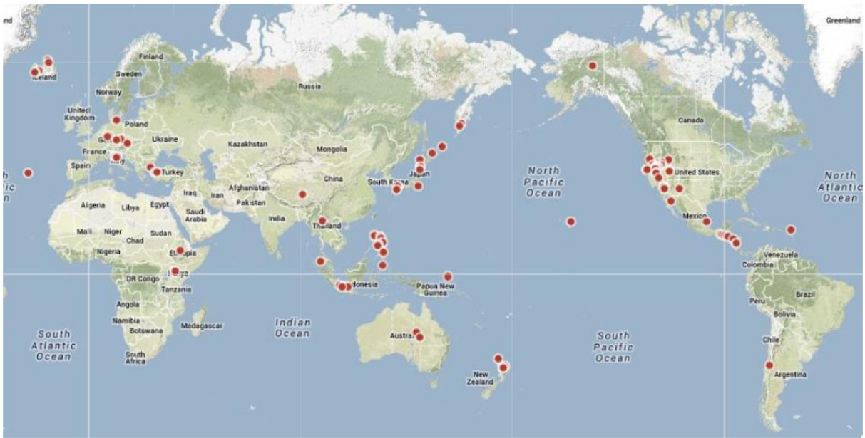
Figure 1.3: Map of the geothermal power plants repartition in the world in 2020 (Huttrer, 2020).
