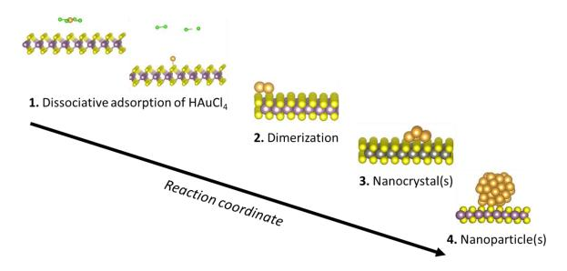
Figure 6-11: Illustration of the principal steps involved in the galvanic displacement reaction leading to the formation of hybrid systems based on  $MS_2$  and AuNPs.
