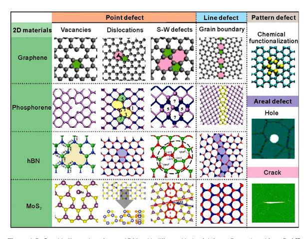
Figure 1-5: Graphic illustration of some 2DMs with different kinds of defects. Reproduced from Ref.<sup>27</sup>.
