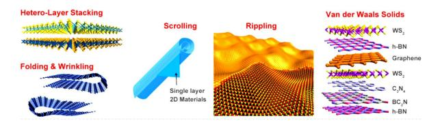
**Figure 3-4**: Schematic illustration of the typical two-dimensional defects encountered in TMDs, such as folding, wrinkling, scrolling, rippling, and vertically stacked heterostructures. Adapted from Ref.<sup>28</sup>.
