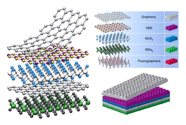
**Figure 1-2**: Fabrication of van der Waals heterostructures. Considering 2D crystals analogous to Lego blocks (right panel), the production of a huge variety of layered structures becomes possible, paving the way for intriguing new opportunities in 2DM science. Reproduced from Ref.<sup>22</sup>.
