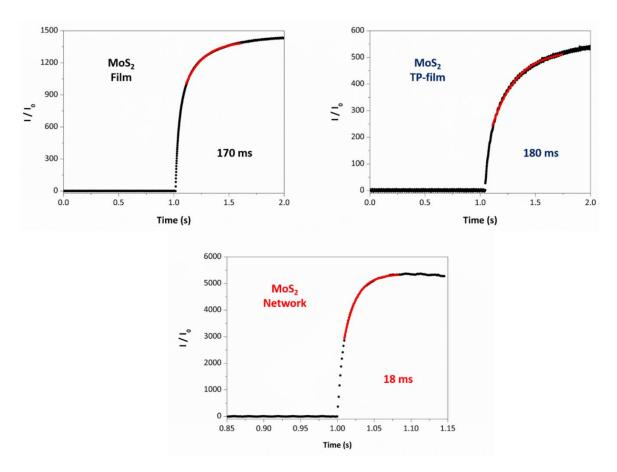
**Figure 5-22**: Current vs. time curves (normalized to starting current  $I_0$ ) for  $MoS_2$  films (black), TP-functionalized films (blue) and networks (red) with related  $\tau_S$ . The red line delimits the range in which a non-linear growth equation can be used to extrapolate  $\tau_S$ .
