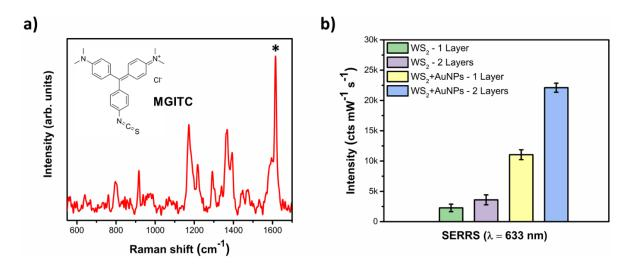
**Figure 6-16 : a)** Raman spectra of MGITC acquired by using a 633 nm laser line. The asterisk shows the peak used for the **b)** SERRS analysis performed on pristine WS<sub>2</sub> and WS<sub>2</sub>/Au hybrid systems.
