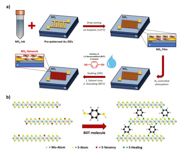
**Figure I : a)** Illustration of the ink deposition and in-situ functionalization to produce  $MS_2$  networks *via* BDT treatment. **b)** Sketch of  $V_S$  healing mechanism in  $MoS_2$  films by means of dithiolated molecules and related inter-flake networking.
