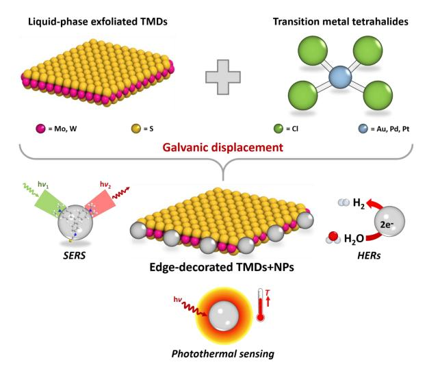
**Figure II:** Illustration of the molecular functionalization strategy adopted for the production of hybrid materials based on solution-processed TMDs and noble metal NPs, whose possible applications are also highlighted (SERS, HERs and photothermal sensing).
