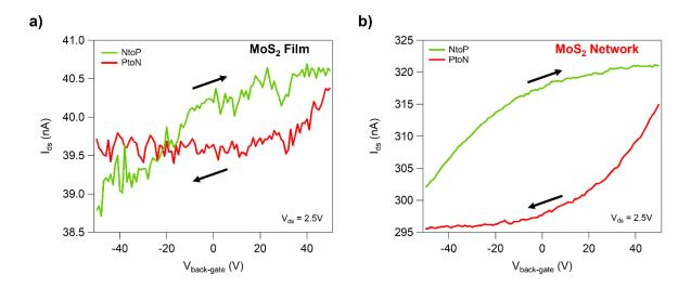
Figure 5-17: Transfer curves for  $MoS_2$  TFTs based on **a)** films and **b)** networks in back-gate configuration. All curves are recorded at  $V_{ds} = 2.5$  V and sweeping  $V_{back-gate}$  from -50 to + 50 V.
