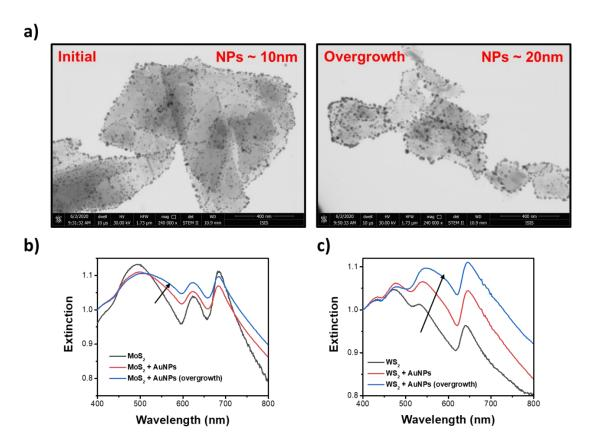
**Figure 6-4 : a)** STEM images, recorded under the same scanning conditions, of  $MoS_2/Au$  hybrid systems at initial condition and after overgrowth reaction. **b)** UV-Vis spectra for  $MoS_2/Au$  and **c)** WS<sub>2</sub>/Au hybrid materials at different steps. The black arrow highlights the plasmon band of AuNPs.
