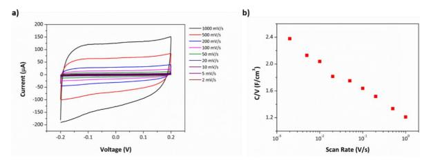
Figure 5-18: a) Cyclic voltammograms recorded for ReS<sub>2</sub> films at different scan rates. b), Scan rate dependence on sample capacitance.
