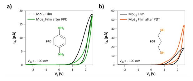
**Figure 5-20**: Transfer curves for  $MoS_2$  LG-TFTs **a)** before and after treatment with PPD and **b)** before and after treatment with PDT. All curves are recorded at  $V_{ds} = -100$  mV, using EMI-TFSI as electrolyte and a Pt wire as gate electrode. The molecular structures of PPD and PDT are indicated.
