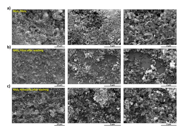
**Figure 5-11 :** SEM images at different magnifications of **a)** MoS<sub>2</sub> pristine films **b)** MoS<sub>2</sub> pristine films after water exposure and **c)** MoS<sub>2</sub> networks after water exposure.
