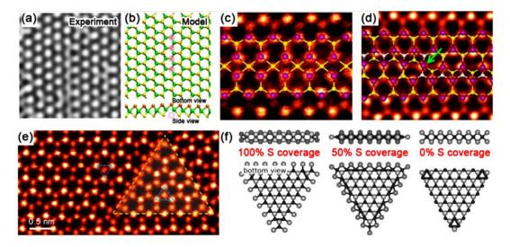
**Figure 3-3**: **a)** HR-TEM image and **b)** structural model showing a single vacancy line in MoS<sub>2</sub> monolayer. **c-d)** ADF images of grain boundaries in CVD MoS<sub>2</sub> monolayers. **e)** ADF image showing an inversion domain in monolayer MoSe<sub>2</sub>. **f)** Structural models showing Mo-terminated MoS<sub>2</sub> domains edges with different percentages of sulfur coverage. Adapted from Ref.<sup>28</sup>.
