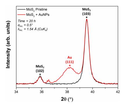
**Figure 6-9 :** GIXD diffractograms (incident angle,  $\alpha_{inc.}$ , 0.5°) of MoS<sub>2</sub> pristine (black) and MoS<sub>2</sub>/Au hybrid materials (red). X-ray wavelength ( $\lambda_{inc.}$ ) = 1.54 Å (Cu<sub>Kα</sub>), scanning time = 20 h.
