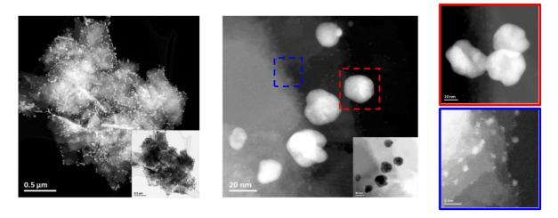
**Figure 6-6 :** HR-TEM images at different magnifications for MoS<sub>2</sub>/Au hybrid materials. The presence of larger and smaller AuNPs at the flake edge is highlighted in red and blue, respectively.
