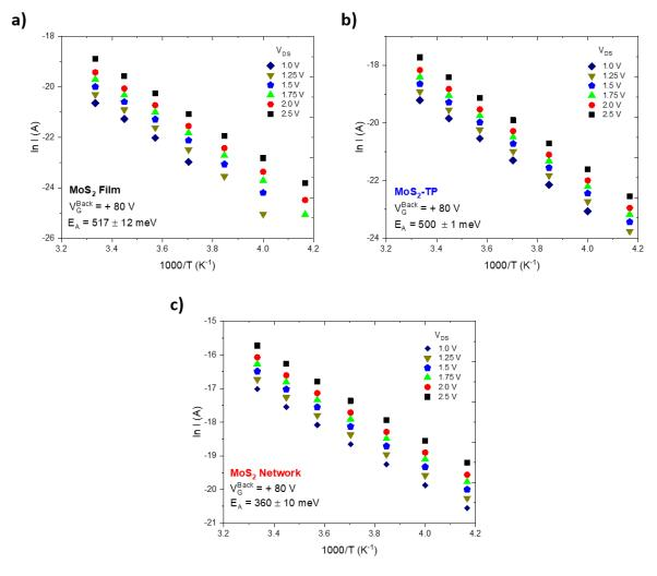
**Figure 5-26**: Ln I vs. 1000/T for  $V_G^{back} = +80 \text{ V}$  in **a)** MoS<sub>2</sub> films **b)** TP-functionalized samples and **c)** MoS<sub>2</sub> networks.  $E_A$  is calculated from the curve slope with errors associated to different applied bias on the IDEs (from 1-2.5 V, *i.e.*,  $E = 4 \times 10^5 - 1 \times 10^6 \text{ V/m}$ ).
