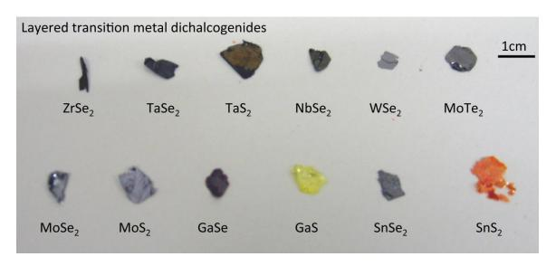
**Figure 2-1**: Photograph displaying the different aspect of bulk crystals for some TMDs. Usually, such systems are employed during the exfoliation procedures performed by micromechanical cleavage using adhesive tape, also known as Scotch-tape approach. Reproduced from the following website: *van-der-waals-epitaxy.info*.
