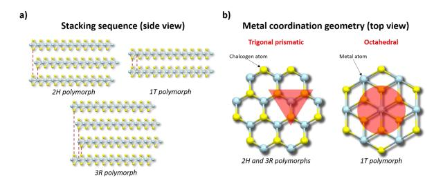
**Figure 2-2**: Illustration of the different polymorph structures for TMDs. **a)** Depiction, in side view, of the three possible TMD polymorphs obtained *via* different stacking sequence of individual layers. **b)** Representation, in top view, of the metal coordination geometry for the three possible TMD polymorphs. Atom color legend: light blue, transition metal atom; yellow, chalcogen atom. Reproduced from Ref.<sup>25</sup>.
