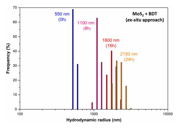
**Figure 5-29**: Hydrodynamic radius of MoS<sub>2</sub> flakes dispersed in IPA and functionalized *ex-situ* with BDT molecules. Each sample is prepared by collecting 500 µl of the ink, successively subjected to 1:100 dilution and sonication/mixing steps.
