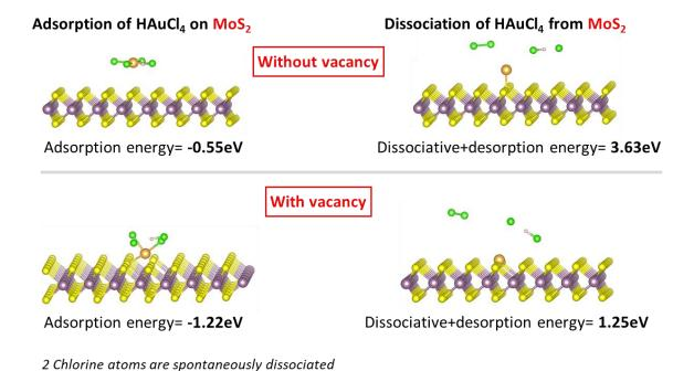
**Figure 6-12 :** Calculation of the adsorption, dissociative and desorption energy for HAuCl<sub>4</sub> on MoS<sub>2</sub>, with and without V<sub>S</sub>.
