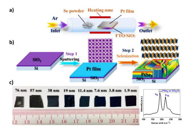
**Figure 2-7**: **a)** Illustration of the growth process for PtSe<sub>2</sub>. **b)** Two-step growth method of PtSe<sub>2</sub> film. Step 1: deposition of Pt film on SiO<sub>2</sub>/Si substrate by magnetron sputtering. Step 2: selenization of the Pt film into PtSe<sub>2</sub>. **c)** As-prepared PtSe<sub>2</sub> films with various thickness (left) and typical Raman spectrum of PtSe<sub>2</sub> film on SiO<sub>2</sub>/Si (right). Adapted from Ref.<sup>58</sup>.
