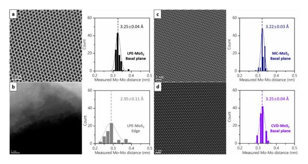
**Figure 5-2 :** HAADF-STEM images and related histograms of Mo-Mo distance for the **a)** basal plane of LPE-MoS<sub>2</sub>, **b)** edge of LPE-MoS<sub>2</sub>, **c)** basal plane of MC-MoS<sub>2</sub> and **d)** basal plane of CVD-MoS<sub>2</sub>. The histograms show a similar average Mo-Mo distance for the basal plane of all samples, with a significant decrease ~30 pm for the edge of LPE-MoS<sub>2</sub>, pointing to a higher defect density.
