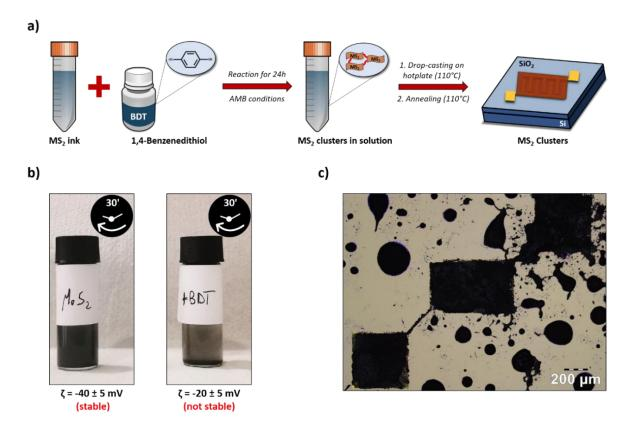
**Figure 5-28 : a)** Schematic illustration for the *ex-situ* functionalization of MS<sub>2</sub> inks with BDT. **b)** Outcome of stability test for pristine and BDT-functionalized MoS<sub>2</sub> ink, along with the related zeta potential values. **c)** Optical image of a IDE device covered with BDT-functionalized MoS<sub>2</sub> ink *via ex-situ* approach.
