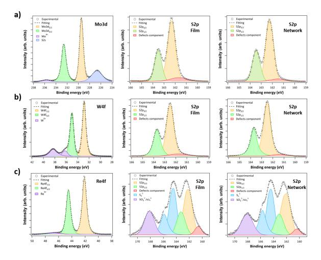
**Figure 5-5 : a)** MoS<sub>2</sub>, with Mo3d (left) and S2p regions, the latter for film (middle) and network (right). **b)** WS<sub>2</sub>, with W4f (left) and S2p regions, the latter for film (middle) and network (right). **c**, ReS<sub>2</sub>, with Re4f (left) and S2p regions, the latter for film (middle) and network (right).
