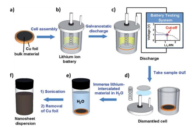
**Figure 2-10**: **a-f)** Illustration of the electrochemical lithium intercalation and exfoliation process to produce 2D nanosheets from layered bulk materials (MN = h-BN, metal selenides, or tellurides in  $Li_xMN$ ). Adapted from Ref.<sup>73</sup>.
