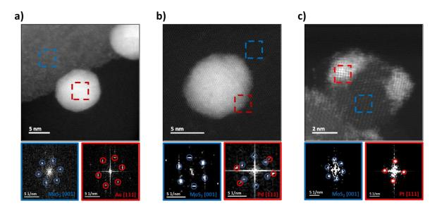
**Figure 6-8 :** HR-TEM and FFT images taken for hybrid systems based on MoS<sub>2</sub> and **a)** Au, **b)** Pd and **c)** PtNPs. The areas where the FFT analysis is performed are highlighted in blue for the 2DMs, while in red for the NPs.
