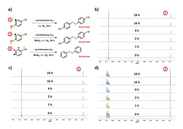
Figure 5-15 : a) Tested reactions between  $MoS_2$  and thiolated molecules under exam (TP and BDT). Related NMR spectra at different time intervals for b) BDT without  $MoS_2$  (control experiment), c)  $MoS_2$  + BDT and d)  $MoS_2$  + TP.
