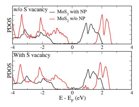
Figure 6-15: PDOS calculated for pristine MoS<sub>2</sub> and MoS<sub>2</sub>/Au hybrid materials, with and without V<sub>S</sub>.
