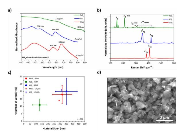
**Figure 4-1 : a)** UV-Vis spectra (solution) and **b)** Raman spectra (film) for solution-processed MS<sub>2</sub>. **c)** Statistical AFM analysis performed on individual MS<sub>2</sub> flakes (300, overall) and comparison with values estimated *via* UV-Vis spectroscopy. **d)** Typical SEM image of drop-cast MoS<sub>2</sub> flakes.
