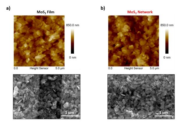
**Figure 5-3**: AFM (top) and SEM (bottom) images for **a)** MoS<sub>2</sub> films and **b)** MoS<sub>2</sub> networks. No significant changes are observed upon BDT functionalization. The SEM images are recorded inbetween Au IDEs of pre-patterned SiO<sub>2</sub>/Si substrates.
