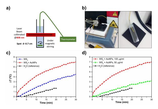
**Figure 6-17 : a)** Sketch and **b)** images of the experimental set-up used for the photothermal analysis. **c)** Photothermal response of pristine  $WS_2$  and hybrid  $WS_2/Au$  compared to water, possessing both a concentration of 100  $\mu$ g/ml. **d)** Photothermal response of hybrid  $WS_2/Au$  systems with different concentration.
