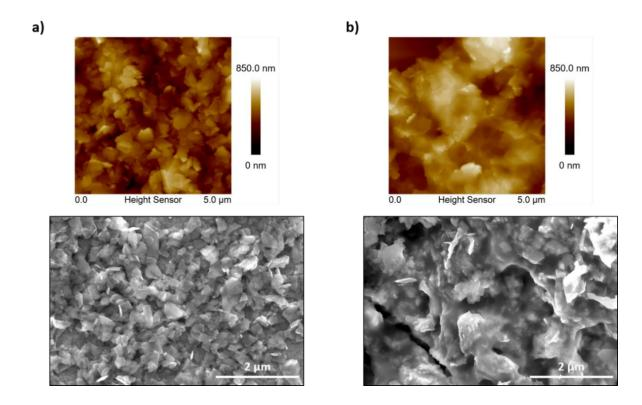
**Figure 5-30 :** AFM (top) and SEM (bottom) images taken for MoS<sub>2</sub> films functionalized **a)** *in-situ* and **b)** *ex-situ* with BDT.
