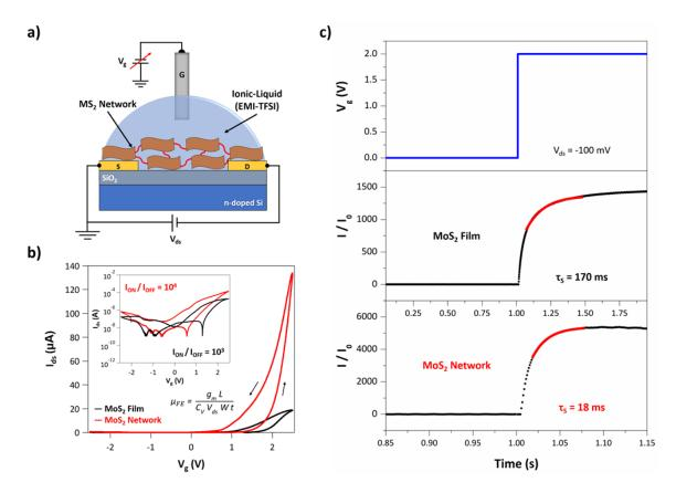
**Figure 5-16 : a)** LG-TFT geometry. **b)** Transfer curves for MoS<sub>2</sub> films and networks with  $V_{ds} = -100$  mV and  $V_g$  sweeping from -2.5 V to +2.5 V. *Inset:* log-scale current characteristics and equation to calculate μ<sub>FE</sub>. **c)** LG-TFT switching characteristics under  $V_g$  step and corresponding time-dependent normalized current response (I/I<sub>0</sub>). The red line delimits the range in which a non-linear fitting can be used to extrapolate  $τ_S$ .
