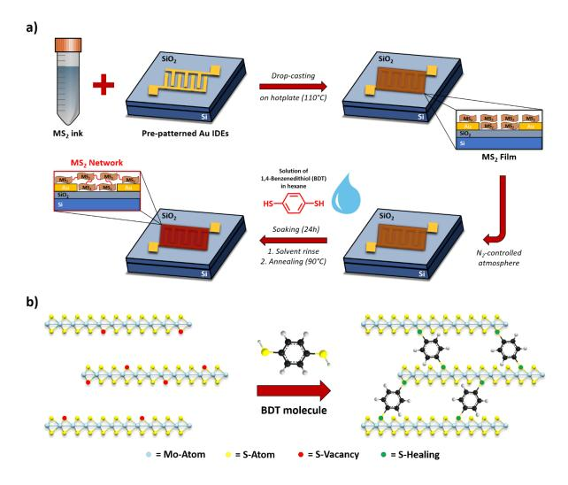
**Figure 5-1 : a)** Illustration of the ink deposition and *in-situ* functionalization to produce  $MS_2$  networks *via* BDT treatment. **b)** Sketch of  $V_S$  healing mechanism in  $MoS_2$  films by means of dithiolated molecules and related inter-flake networking.
