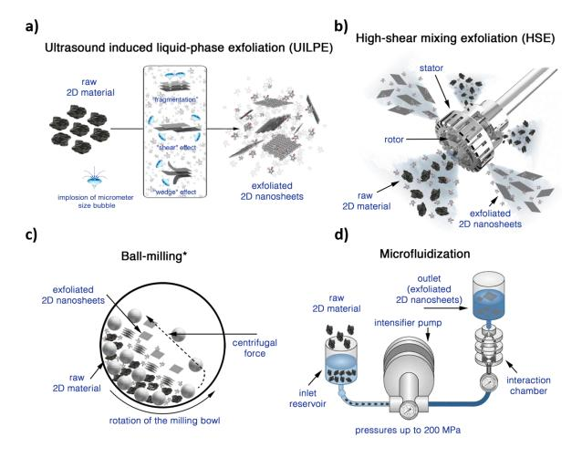
**Figure 2-11**: Schematic representation of various LPE-based methods, such as **a)** ultrasound-induced LPE, **b)** high-shear mixing exfoliation, **c)** ball milling, **d)** microfluidization. Adapted from Ref.<sup>77</sup>.
