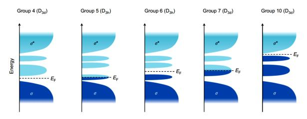
**Figure 2-3**: Schematic illustration showing the progressive filling of the *d* bands located between the bonding ( $\sigma$ ) and anti-bonding ( $\sigma^*$ ) states in group 4, 5, 7, and 10 TMDs. D<sub>3h</sub> and D<sub>3d</sub> indicate the point groups matching the 1H and 1T polymorphs, respectively. Reproduced from Ref.<sup>41</sup>.
