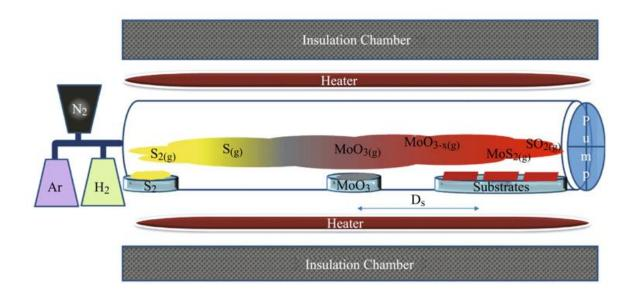
Figure 2-6: Sketch of a CVD reactor for the production of MoS<sub>2</sub> nanosheets. Reproduced from Ref.<sup>55</sup>.
