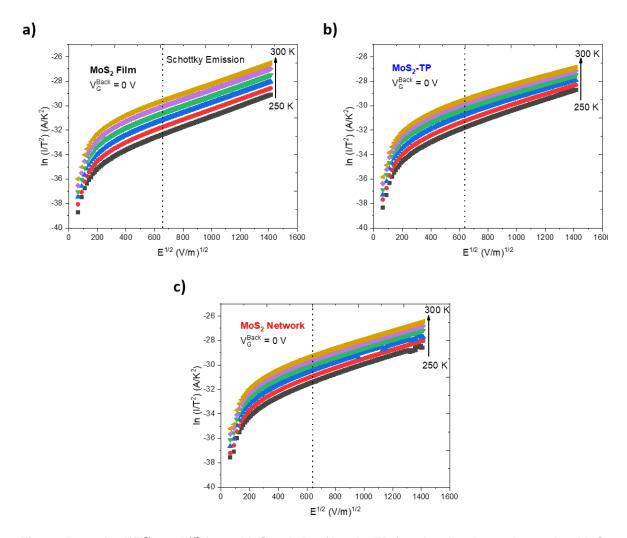
**Figure 5-24**: Ln I(/T²) vs.  $E^{1/2}$  for **a**, MoS₂ pristine films **b**, TP-functionalized samples and **c**, MoS₂ networks in a T range 250-300 K without an external gate bias on the back electrode of Si/SiO₂/IDE test patterns.
