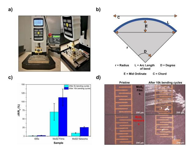
**Figure 5-12 : a)** Experimental setup. **b)** Sketch of the samples subjected to bending deformation. **c)** Variation of the relative channel resistance  $\Delta R/R_0$  of bare IDEs, MoS<sub>2</sub> films, and MoS<sub>2</sub> networks upon 5k and 10k bending cycles, along with related **d)** optical images of MoS<sub>2</sub> films and networks before (left) and after (right) mechanical deformation.
