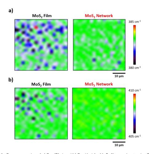
**Figure 5-9 :** Raman mapping of **a)**  $Pos(E^{1}_{2g})$  and **b)**  $Pos(A_{1g})$  for  $MoS_{2}$  films and networks. Each map contains 441 spectra and covers 1600  $\mu m^{2}$ .
