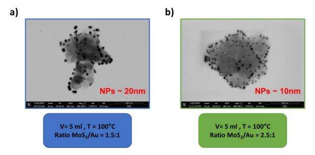
**Figure 6-1 :** STEM images, recorded under the same scanning conditions, of MoS<sub>2</sub>/Au hybrid materials synthesized with **a)** 1.5:1 and **b)** 2.5:1 concentration ratio.
