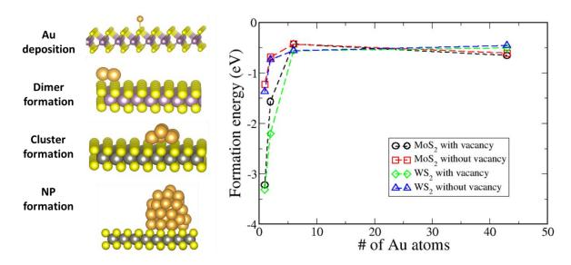
**Figure 6-14 :** DFT calculations of the formation energy of Au clusters on  $MoS_2$  and  $WS_2$  as a function of the number of constituent Au atoms. The very same calculations are carried out in presence and absence of  $V_S$ .
