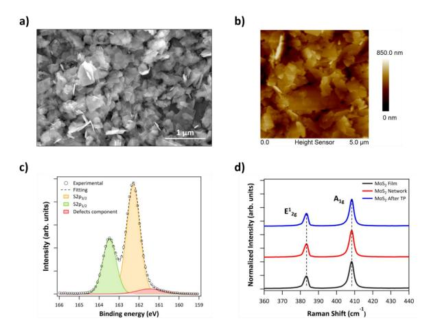
**Figure 5-13 : a)** SEM image, **b)** AFM image and **c)** HR-XPS S2p spectrum of MoS<sub>2</sub> upon TP exposure. **d)** Raman spectra of MoS<sub>2</sub> films, networks and TP-functionalized films.
