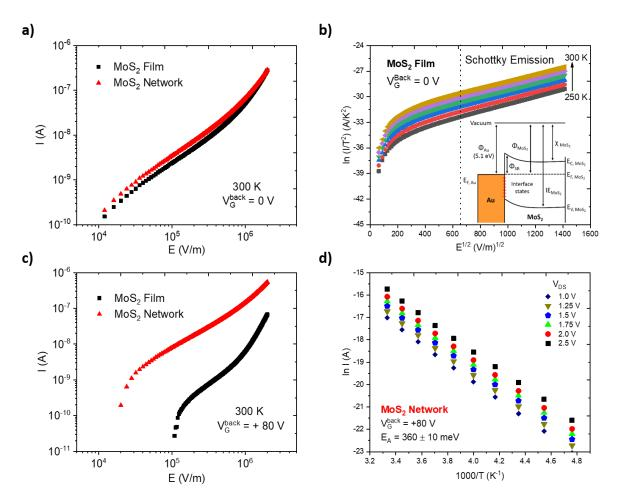
**Figure 5-23 : a)** 300K I-E curves for  $V_G^{Back} = 0$  for  $MoS_2$  films (black) and networks (red). **b)** Schottky plot for  $MoS_2$  film for  $V_G^{Back} = 0$  V. *Inset*: Band diagram for Au/MoS<sub>2</sub> Schottky barrier interface. **c)** 300K I-E characteristic with for  $V_G^{Back} = +80$  V in  $MoS_2$  films (black) and networks (red). **d)** Arrhenius plot for  $MoS_2$  network for  $V_G^{Back} = +80$  V.
