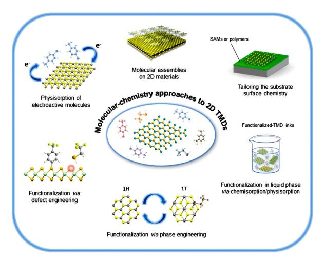
**Figure 1-3**: Schematic representation of the different molecular chemistry approaches that have been investigated in the last few years for tailoring the properties of 2D TMDs. Reproduced from Ref.<sup>8</sup>.
