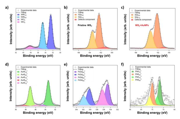
**Figure 6-10**: HR-XPS spectra recorded in different regions, namely **a)** W4f, **b)** S2p for pristine and **c)** hybrid materials, **d)** Au4f, **e)** Pd3d and **f)** Pt4f.
