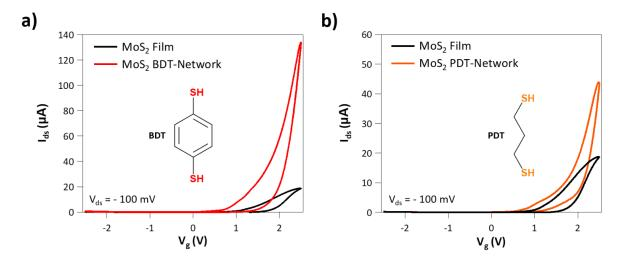
**Figure 5-21 :** Transfer curves for  $MoS_2$  LG-TFTs **a)** before and after treatment with BDT linkers and **b)** before and after treatment with PDT linkers. All curves are recorded at  $V_{ds}$  = -100 mV, using EMI-TFSI as electrolyte and a Pt wire as gate electrode. The molecular structures of BDT and PDT are also indicated.
