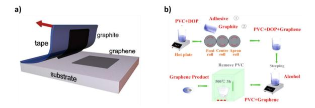
**Figure 2-9: a)** Cartoon illustrating the mechanical exfoliation process of graphite to obtain graphene. **b)** Schematic illustration of the approach used to exfoliate natural graphite by three-roll mill. Reproduced from Ref.<sup>70</sup>.
