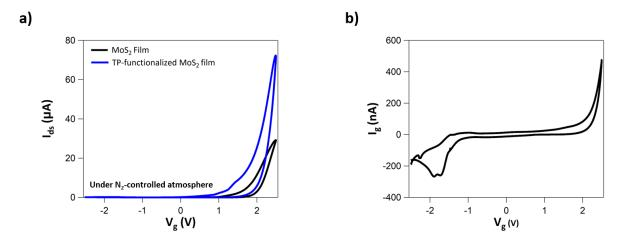
**Figure 5-19 : a)** Comparison between two typical transfer curves for pristine  $MoS_2$  (black) and TP-functionalized  $MoS_2$  (blue) films. **b)** Typical leakage curve for  $MoS_2$  LG-TFTs. All curves are recorded for  $V_{ds}$  = -100 mV and sweeping  $V_g$  from -2.5 to +2.5 V.
