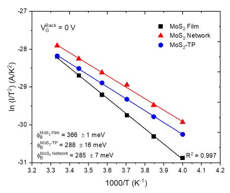
**Figure 5-25**:  $\Phi_B$  calculated from the Schottky formalism for MoS<sub>2</sub> pristine films, TP-functionalized samples and MoS<sub>2</sub> networks. The errors in  $\Phi_B$  correspond to the standard deviation of values calculated at different E.
