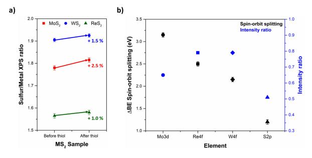
**Figure 5-7 : a)** Sulfur/Metal XPS ratio before and after exposure to BDT molecules for MoS<sub>2</sub>, WS<sub>2</sub> and ReS<sub>2</sub>. **b)** Summary of the XPS constraints (spin-orbit splitting and intensity ratio) implemented for the fitting of Mo3d, Re4f, W4f and S2p regions, before and after exposure to BDT molecules.
