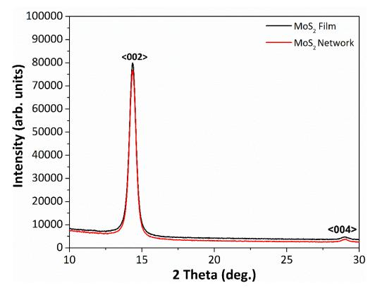
**Figure 5-4**: Comparison of MoS<sub>2</sub> diffractograms obtained for films (black) and networks (red), displaying the characteristic peaks related to the (002) and (004) crystallographic planes.
