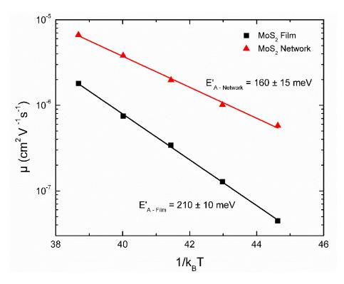
**Figure 5-27 :** Mobility Arrhenius plots for electrical devices based on  $MoS_2$  films and networks in back-gated configuration. The mobility is extracted from the transfer curves for  $V_{ds} = 5$  V and sweeping  $V_{G}^{back}$  from -60 to +60 V.
