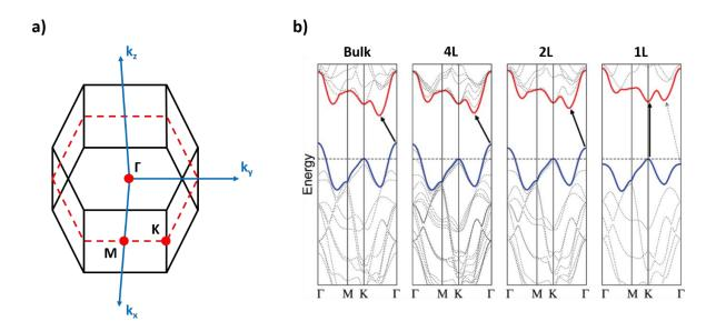
**Figure 2-4**: **a)** Brillouin zone of  $MoS_2$  highlighting the high-symmetry points in the hexagonal lattice. In particular,  $\Gamma$  represents the centre of the Brillouin zone; M describes the centre of a rectangular face; K represents the middle of an edge joining two rectangular faces. **b)** Evolution of the band structure of  $MoS_2$  with decreasing thickness. From left to right: bulk crystal, four-layer (4L), bilayer (2L), and monolayer (1L). Reproduced from Ref.<sup>43</sup>.
